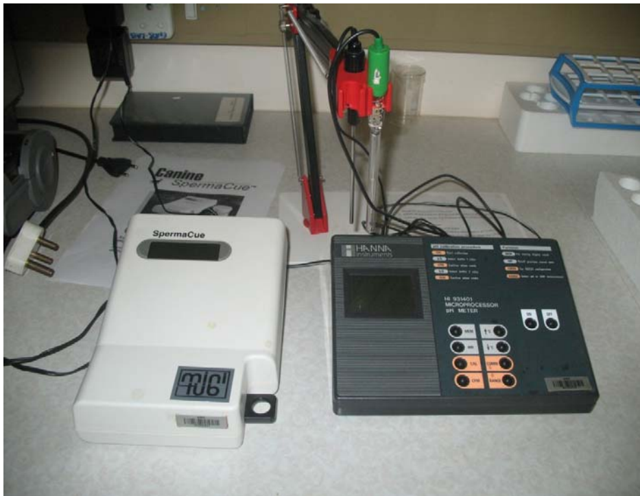
Plate 3.9 A spectrophotometer and the pH meter used in semen evaluation
