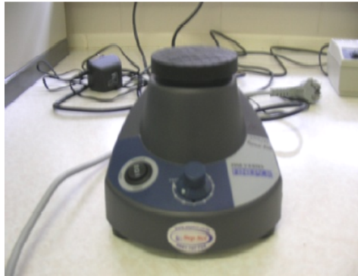
Plate 3.2 A vortexing device for stripping off of cumulus cells
