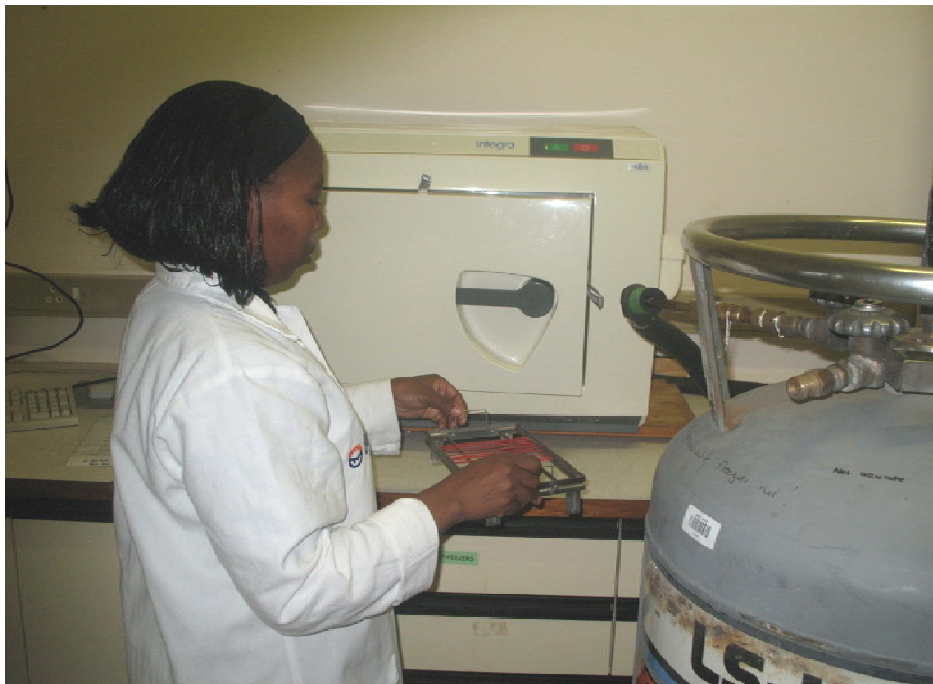
Plate 3.10 Placing of loaded straws into a programmable freezer
