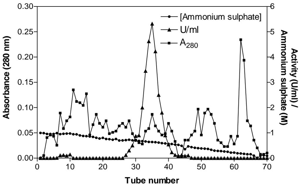
**Figure 4.15.** Phenyl Toyopearl elution profile of the pooled fraction collected from CM Toyopearl. Pooled fraction = 32 - 38.
