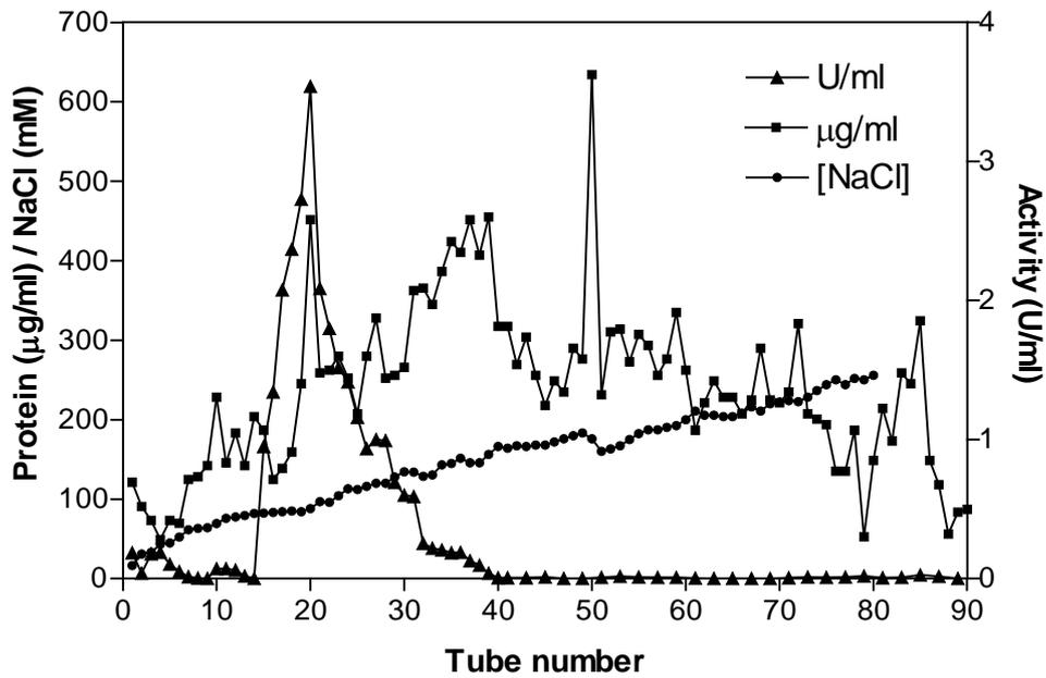
**Figure 4.6.** Super-Q Toyopearl elution profile of the soluble (cytoplasmic) ferric reductase. Pooled fraction = 15 - 25.
