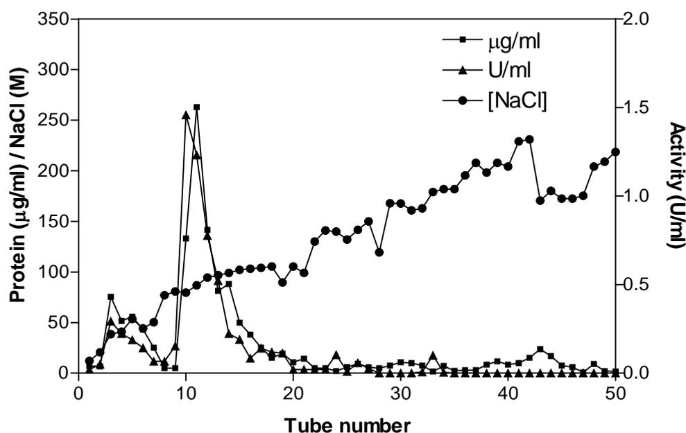
**Figure 4.16.** Super-Q Toyopearl elution profile of the extracted membrane-associated ferric reductase. Pooled fraction = 10 – 17.
