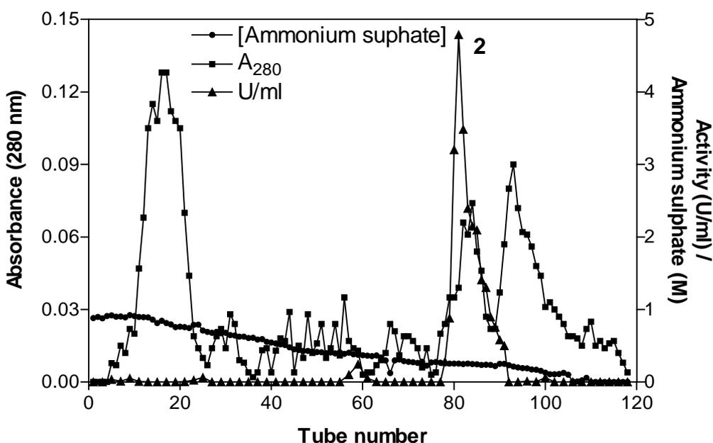
**Figure 4.12.** Phenyl Toyopearl elution profile of Fraction 1 collected from CM Toyopearl. Pooled fraction = 82-85.
