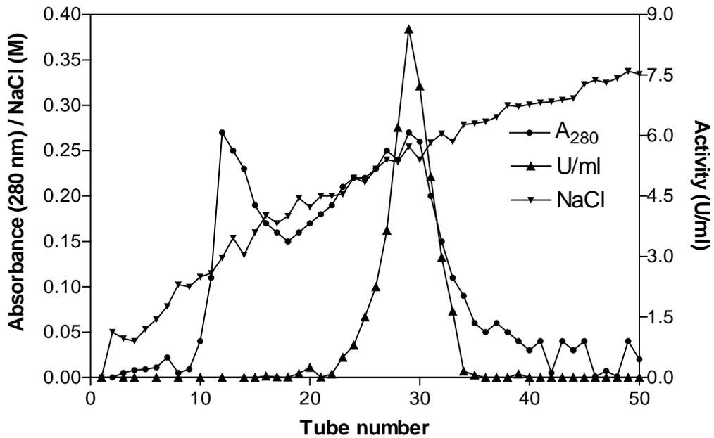
**Figure 4.14.** CM Toyopearl elution profile of the soluble (cytoplasmic) ferric reductase. Pooled fraction = 25 - 33.
