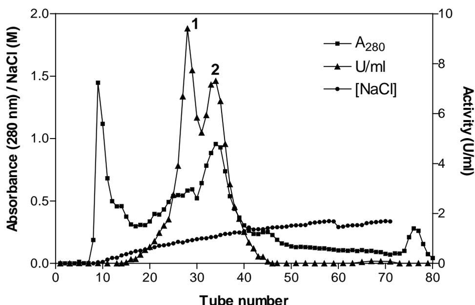
**Figure 4.10.** CM Toyopearl elution profile of the soluble (cytoplasmic) ferric reductase. Pooled fraction 1 = 25 - 31. Pooled fraction 2 = 32 - 38.
