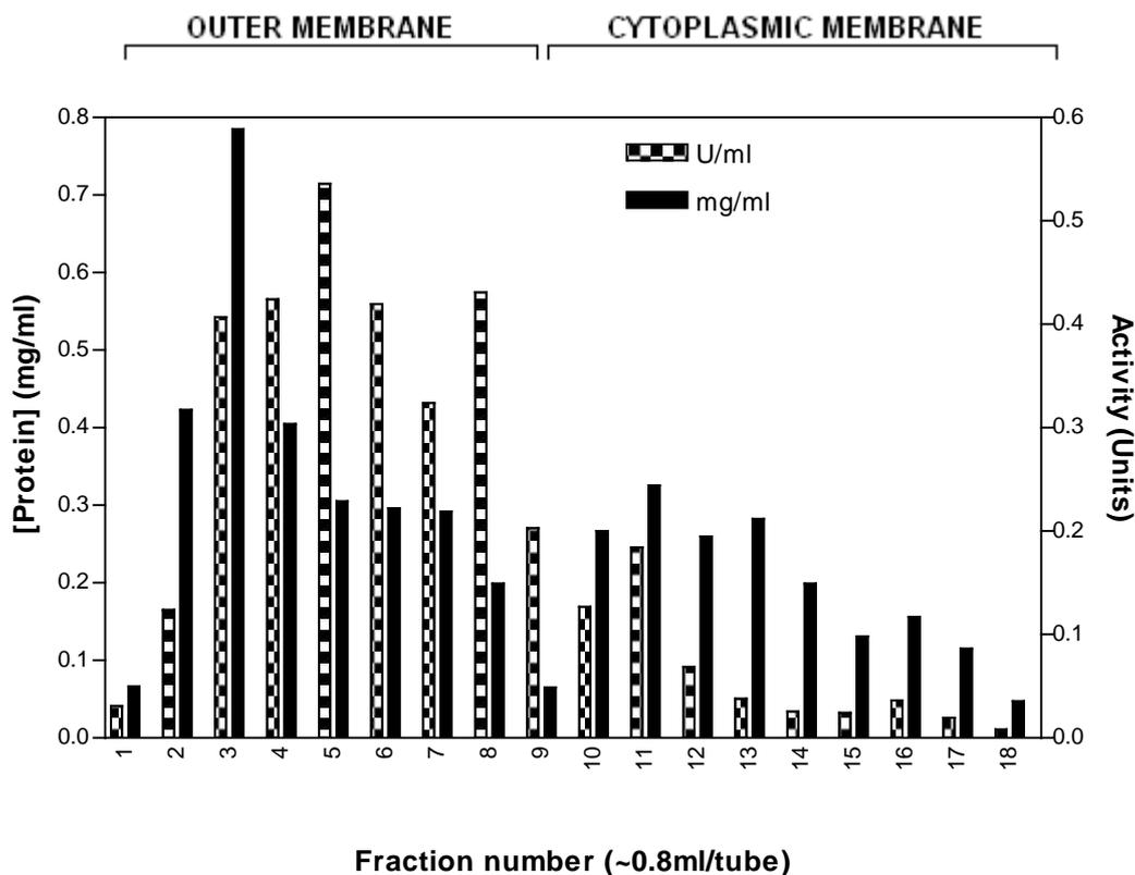
**Figure 4.5.** Highly concentrated sucrose gradient separation of the outer and cytoplasmic membranes for evaluation of the ferric reductase distribution in the membrane fraction.
