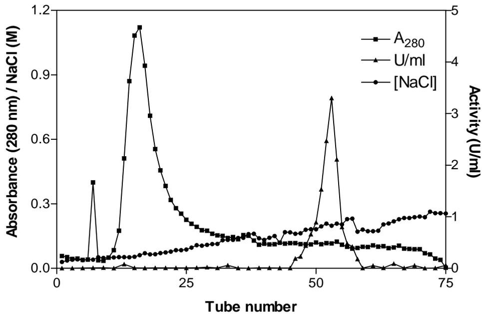
**Figure 4.8.** CM Toyopearl elution profile of the soluble (cytoplasmic) ferric reductase. Pooled fraction = 47 - 58.
