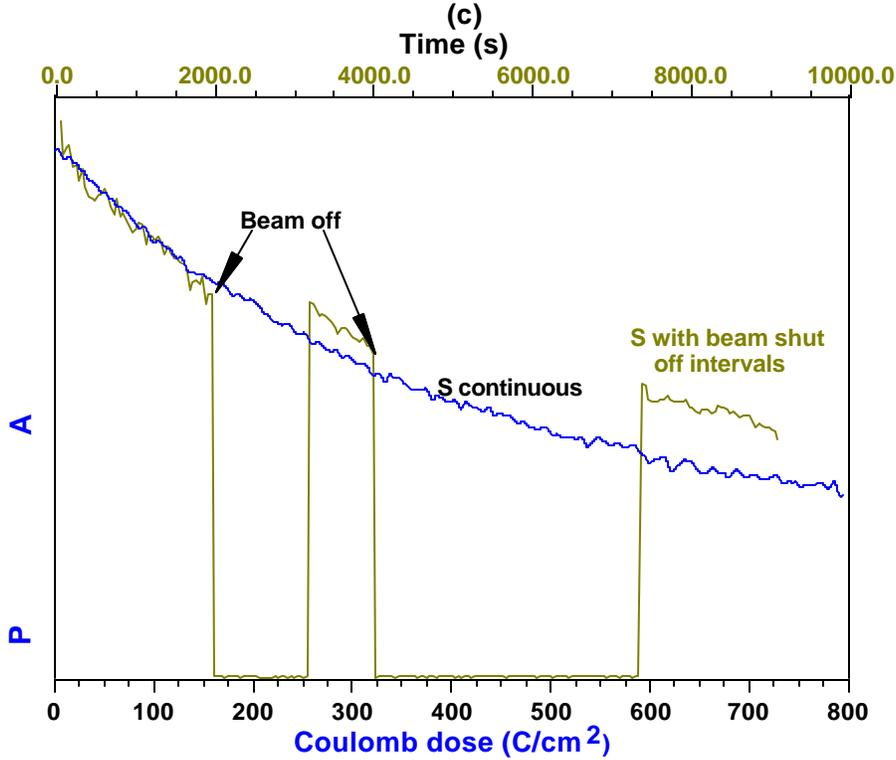
**Figure 5.3 (c) APPHs of S as a function of Coulomb dose and time for continuous bombardment and with beam shut off intervals, as indicated, measured at a current density of 88 mA/cm<sup>2</sup> at a temperature of 260 °C, after sputtering.**
