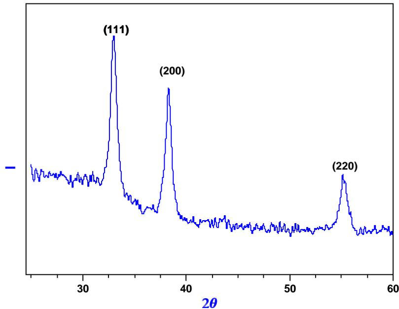
**Figure 8.1 XRD spectrum of CdO bulk precipitate on a glass substrate.**
