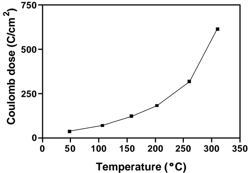
**Figure 5.4 The Coulomb doses required to reach 60% of the original S signal as function of temperature**
