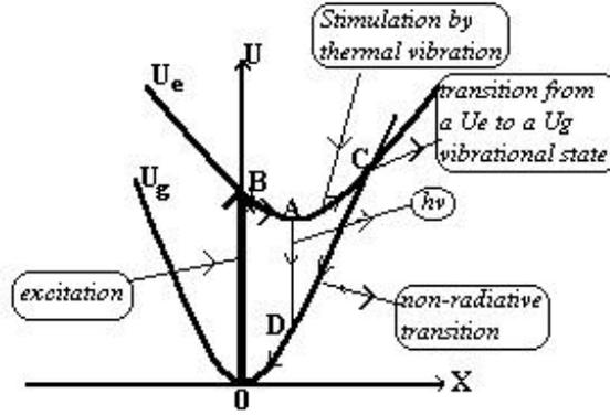
**Figure 2.3 Configuration co-ordinate model of a luminescent centre. The potential energy of a luminescent centre is presented as a function of a generalised co-ordinate  $x$  with the parabolas,  $U_g$  and  $U_e$ , corresponding to the ground and excited states, respectively.**
