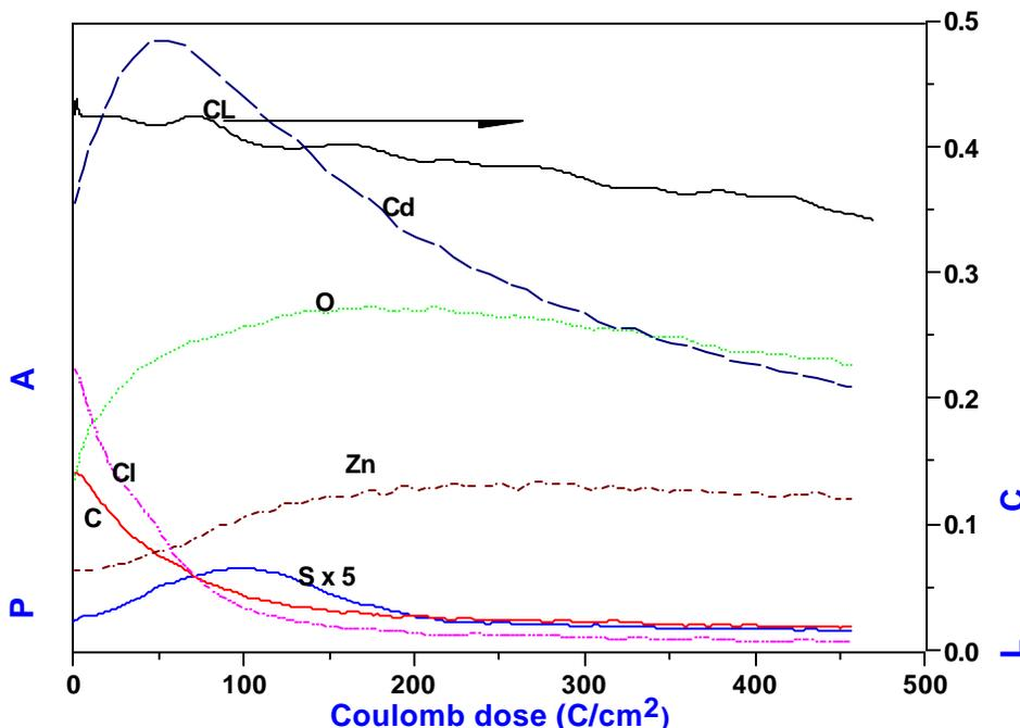
**Figure 8.4** APPHs of Cd, O, C, S, Cl and Zn as well as the CL measured during degradation in an O<sub>2</sub> ambient as function of Coulomb dose.
