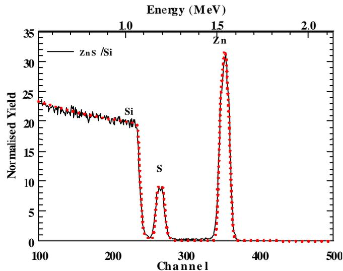
**Figure 6.1** RBS spectrum of pulsed laser deposited ZnS phosphor film on Si(100), the dotted line is the ZnS 1:1 compositional simulation.
