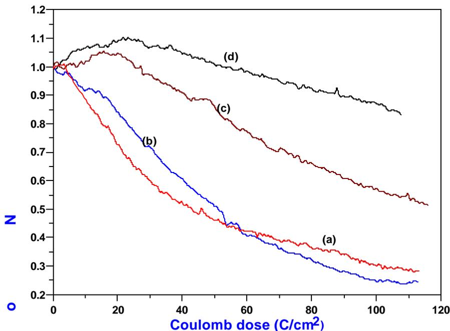
**Figure 9.1 Normalised S APPHs as a function of Coulomb dose acquired at (a) room temperature without cooling, (b) at  $-125\text{ }^{\circ}\text{C}$  without cooling, (c)  $-125\text{ }^{\circ}\text{C}$  with cooling and (d) room temperature with cooling.**
