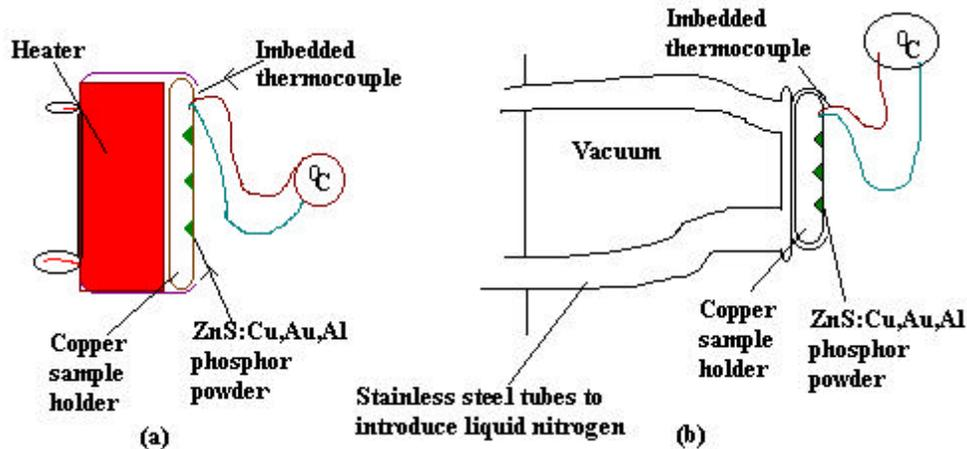
**Figure 3.1** The cross sectional schematics of the heating (a) and cooling (b) set-ups.
