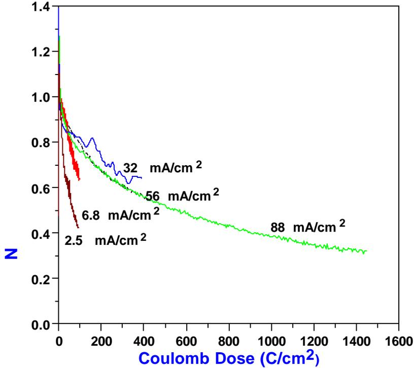
**Figure 4.4** Normalised CL intensities measured at different electron current densities as a function of Coulomb dose.
