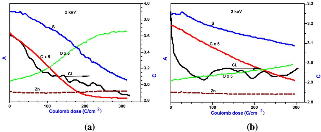
**Figure 7.2** The APPH of S, C, O, and Zn as well as the CL measured during degradation in a  $5 \times 10^{-7}$  Torr O<sub>2</sub> ambient (a) and a  $5 \times 10^{-7}$  Torr CO<sub>2</sub> ambient (b) as a function of Coulomb dose.
