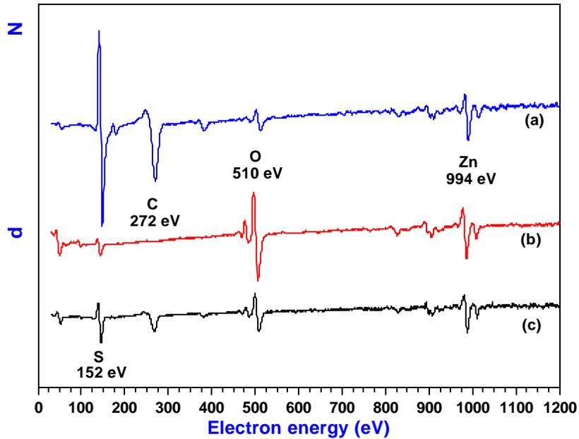
**Figure 7.1** AES differential energy spectra of (a) film before degradation, (b) and (c) film after degradation for a Coulomb dose of about  $300 \text{ C/cm}^2$  in  $\text{O}_2$  and  $\text{CO}_2$ , respectively.
