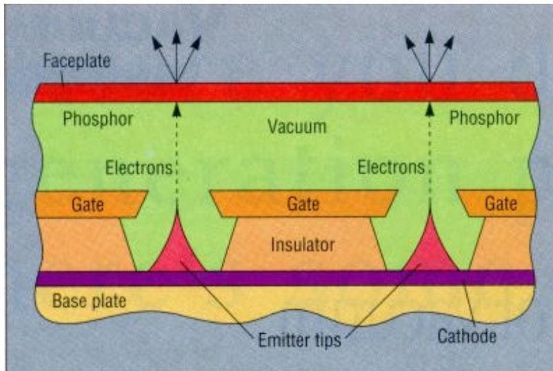
**Figure 1.1 shows the cross-sectional view of the field emission cathodes (FED) [9].**
