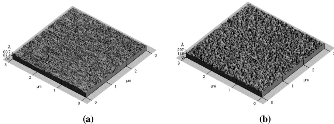
**Figure 6.4** Three-dimensional AFM images of the ZnS films deposited on Si (100), (a) Sample 1 and (b) Sample 4.
