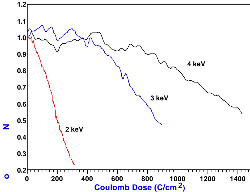
**Figure 7.3** Normalised APPH of sulphur for different electron beam energies as a function of Coulomb dose at an  $O_2$  pressure of  $5 \times 10^{-7}$  Torr.
