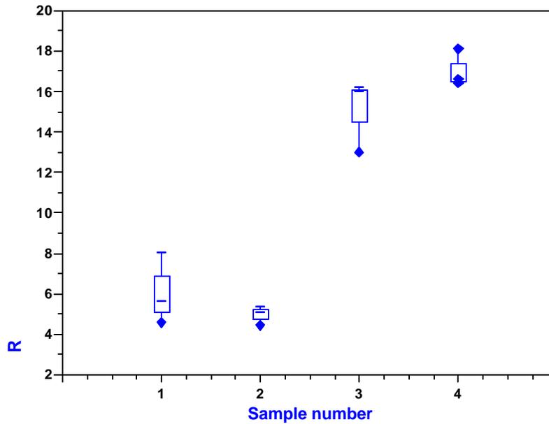
**Figure 6.5** The statistical presentation of calculated rms roughness ( $R_{\text{rms}}$ ) values for all the films.
