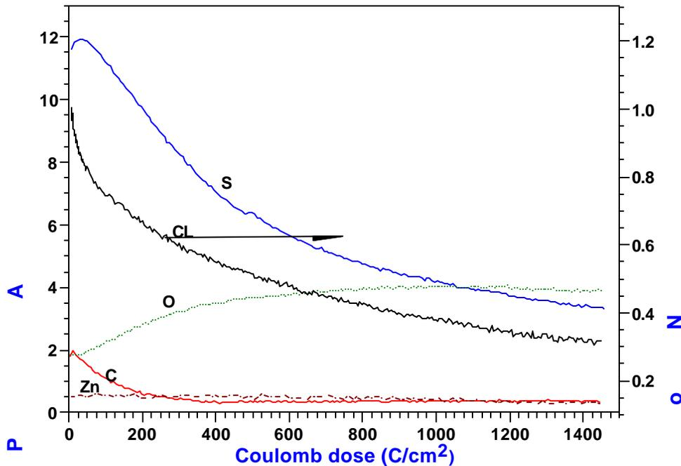
**Figure 4.1** The APPHs of S, C, O and Zn as well as the CL measured at a current density of  $88 \text{ mA/cm}^2$  as a function of Coulomb dose.
