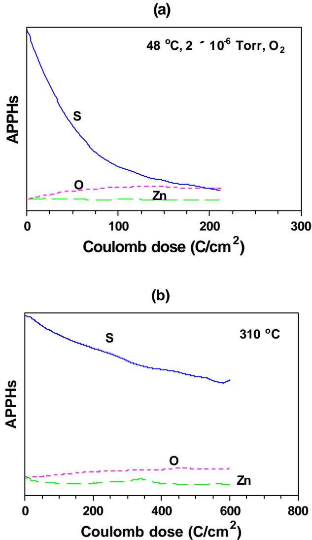
**Figure 5.3** APPH of S, O and Zn as a function of Coulomb dose measured at a current density of 88 mA/cm<sup>2</sup> at temperatures of (a) 48 °C and (b) 310°C, as indicated, after sputtering.
