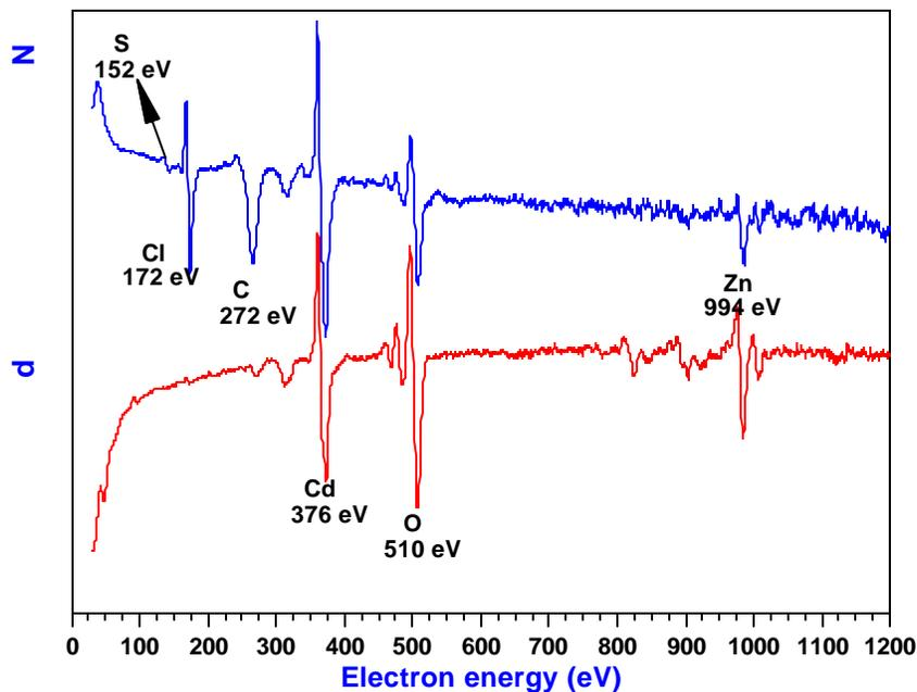
**Figure 8.3** Auger spectra before and after degradation in an  $O_2$  ambient for  $470 C/cm^2$ .
