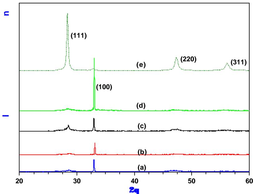
**Figure 6.7** XRD spectra of the films, (a) sample 1, (b) sample 2, (c) sample 3, (d) sample 4 and (e) spectrum of the target material.
