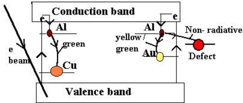
**Figure 2.2** The schematic presentation of the luminescence process in ZnS:Cu,Al,Au phosphor
