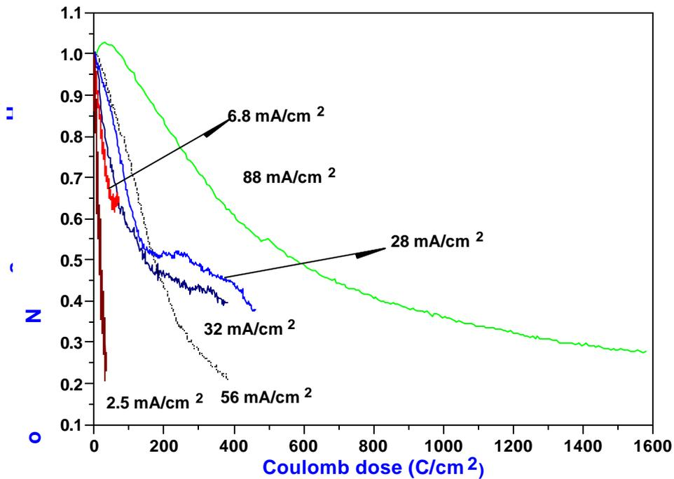
Figure 4.3 Normalised APPHs of sulphur at different electron current densities as a function of Coulomb dose.
