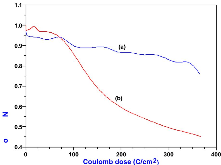
**Figure 8.5 Normalised CL intensity measured during degradation for (a) coated and (b) bare ZnS:Cu,Au,Al thin film phosphor as a function of Coulomb dose.**
