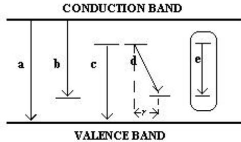
**Figure 2.1 Models of electron transitions resulting in luminescence (a) From conduction band to a hole in the valence band; (b) from a conduction band to an acceptor level; (c) from a donor level to a hole in the valence band; (d) from a donor level to an acceptor level; (e) within a localised luminescent centre.**
