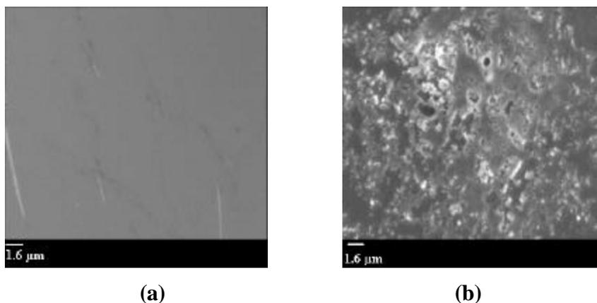
**Figure 8.2 SEM images of a ZnS:Cu,Au,Al thin film (a) and a CdO coated ZnS:Cu,Au,Al thin film (b).**
