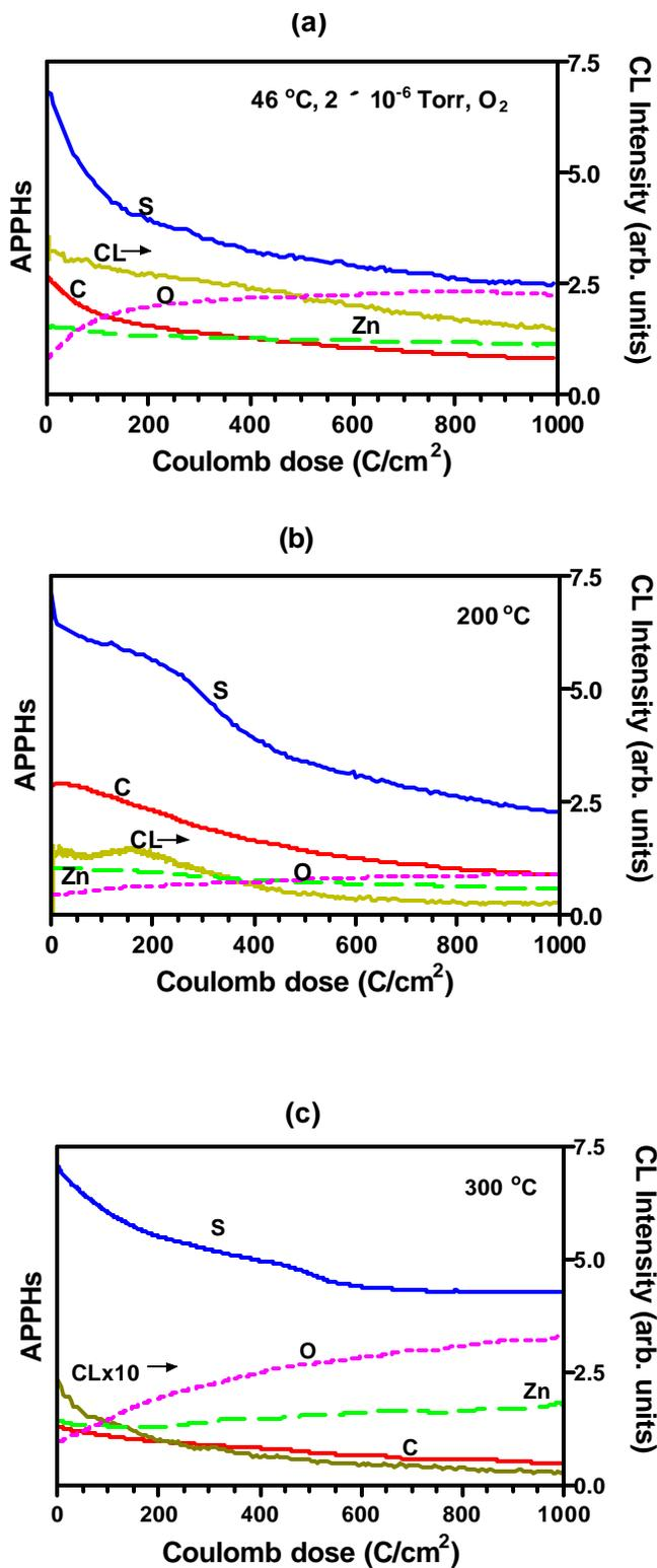
Figure 5.1 APPHs of S, C x 5, O and Zn as well as the CL as a function of Coulomb dose measured at a current density of 88 mA/cm<sup>2</sup> at temperatures of (a) 46 °C, (b) 200 °C and (c) 300 °C as indicated.
