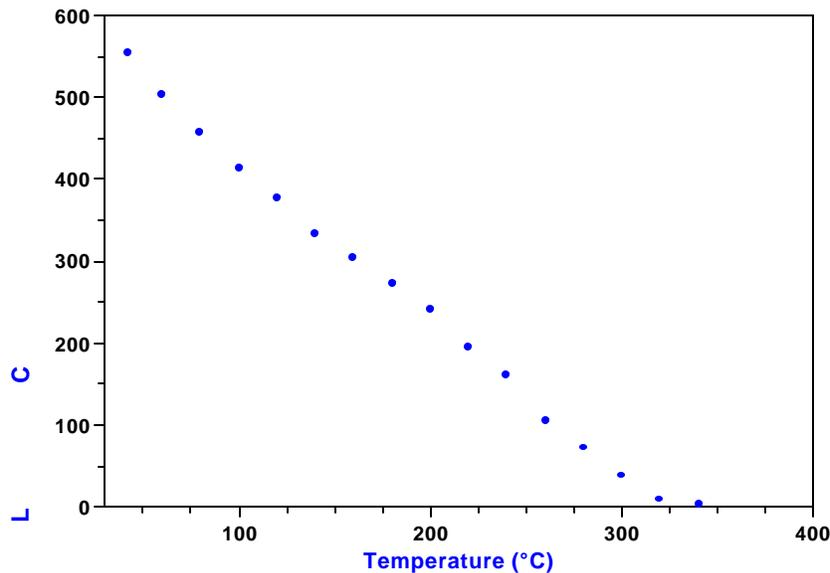
**Figure 5.2** The CL intensity as function of temperature at a pressure of  $2 \times 10^{-9}$  Torr before any degradation.
