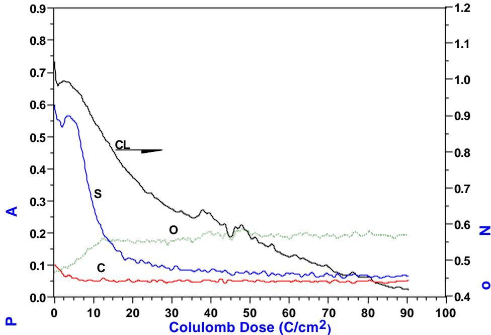
Figure 4.2 The APPHs of S, C, O and Zn as well as the CL measured at a current density of 2.5 mA cm<sup>-2</sup> as a function of Coulomb dose.
