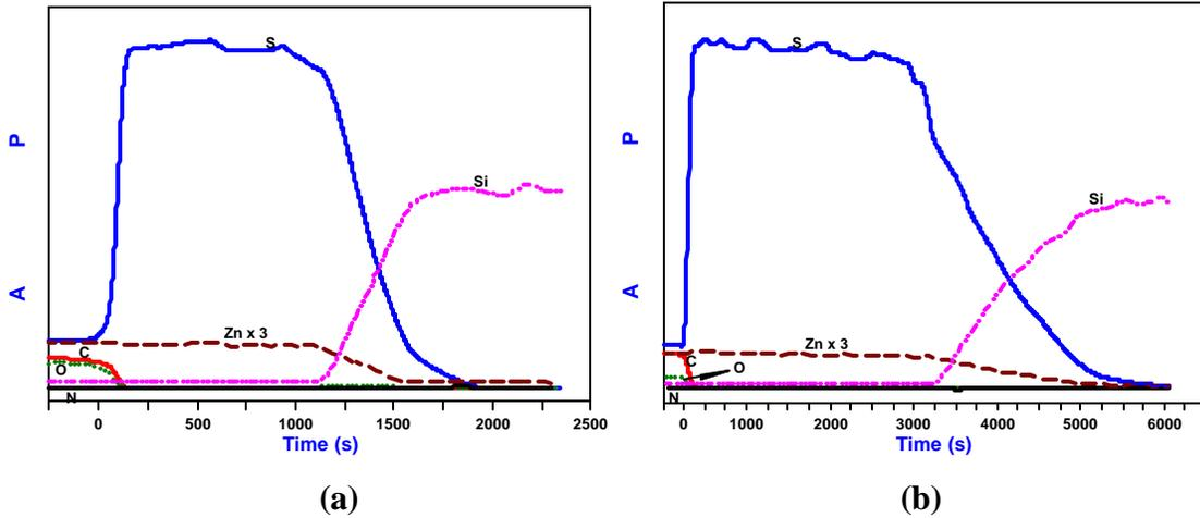
**Figure 6.3** AES depth profiles of (a) sample 1 and (b) sample 4.
