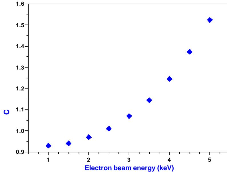
**Figure 7.4 CL intensity at different electron beam energies.**
