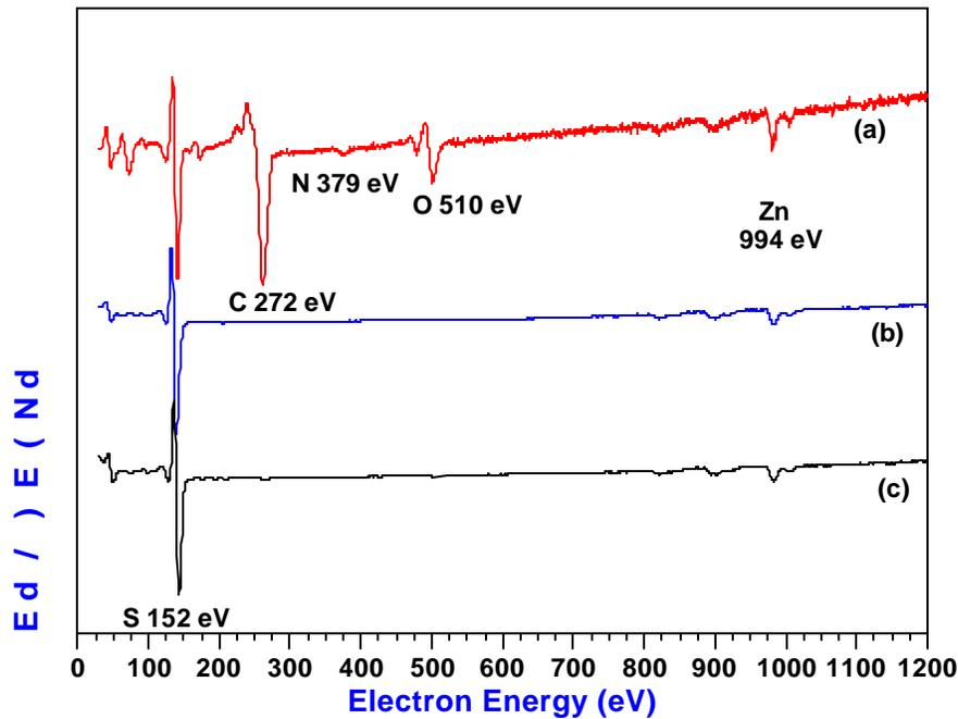
**Figure 6.2** AES differential energy spectra of (a) first layer before sputtering, (b) sample 1 and (c) sample 4, both during sputtering.
