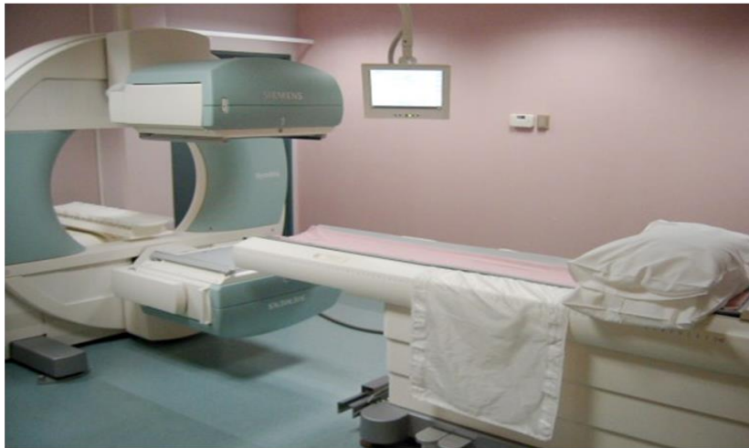
Figure 2-2: (A) The different components of a gamma camera detector. (B) A dual head SPECT gamma camera mounted on a rotating gantry.
