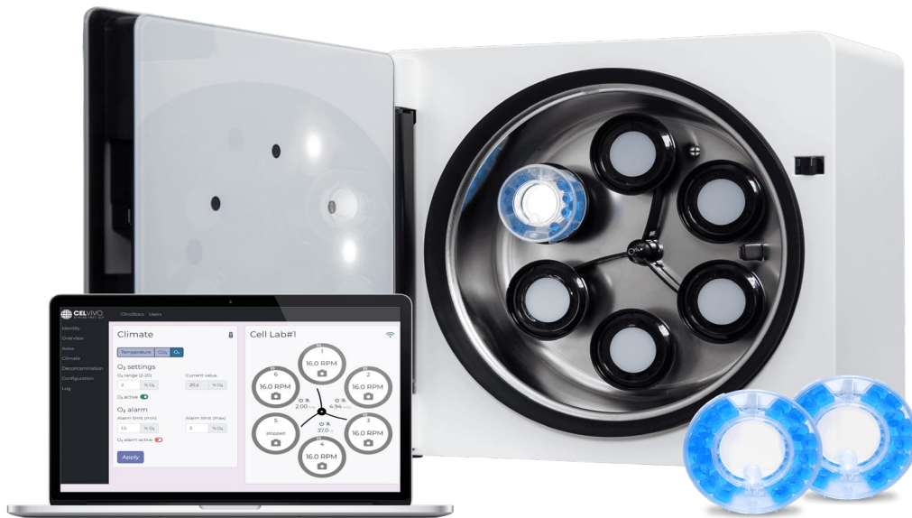
Figure 8. The CelVivo™ ClinoStar™ System, with the ClinoReactors™, used for culturing spheroids in a growth medium. An internet-connected device controls the system's conditions, such as temperature range, carbon dioxide levels, and rotation speed. It visualizes the growing spheroids without opening the system and retrieving the ClinoReactors™ (Taken from the CelVivo™ website, 21 June 2024).
