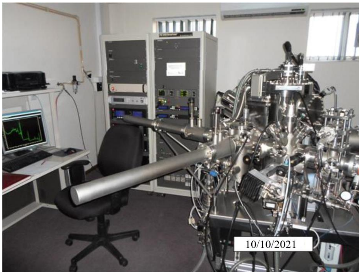
Figure 4.18: PHI 5000 Versaprobe XPS system at the Department of Physics, University of the Free State.
