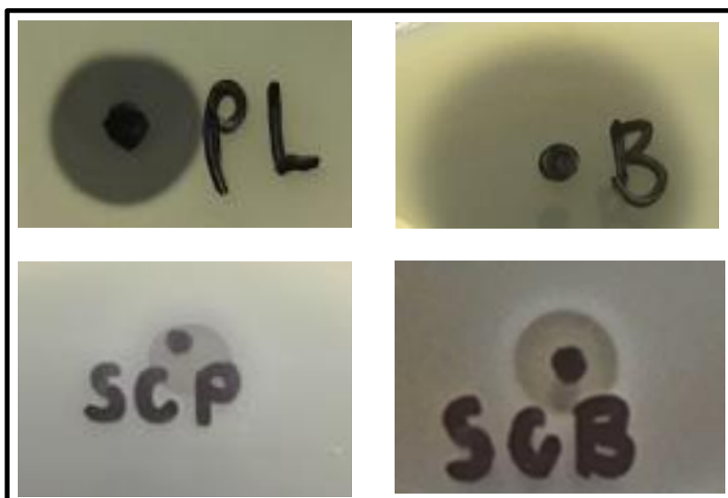
Figure 3.10. Milk agar plates containing commercial Plasmin (indicated by PL), commercial Bacillus protease (indicated by B), the self-produced Pseudomonas protease is indicated by SCP and the self-produced Bacillus protease is indicated by SCB.
