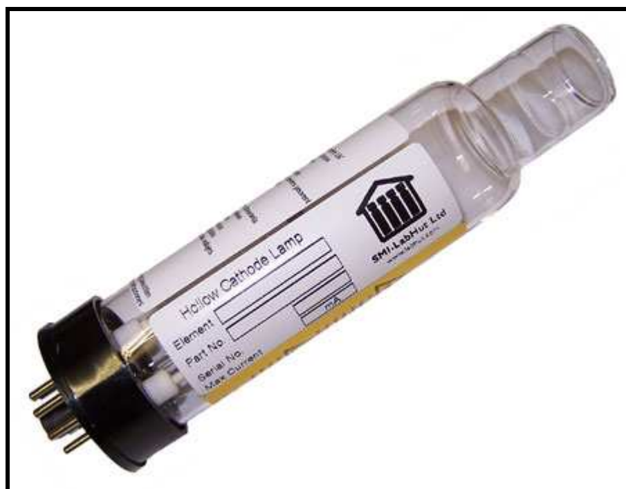
Figure 3.11: A Hollow cathode lamp for Nb 69
