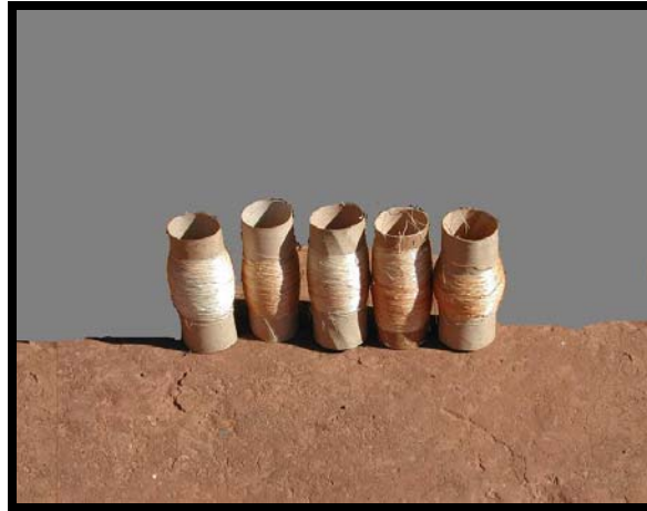
Figure 3.5 Reeled decorticated Agave americana fibres
