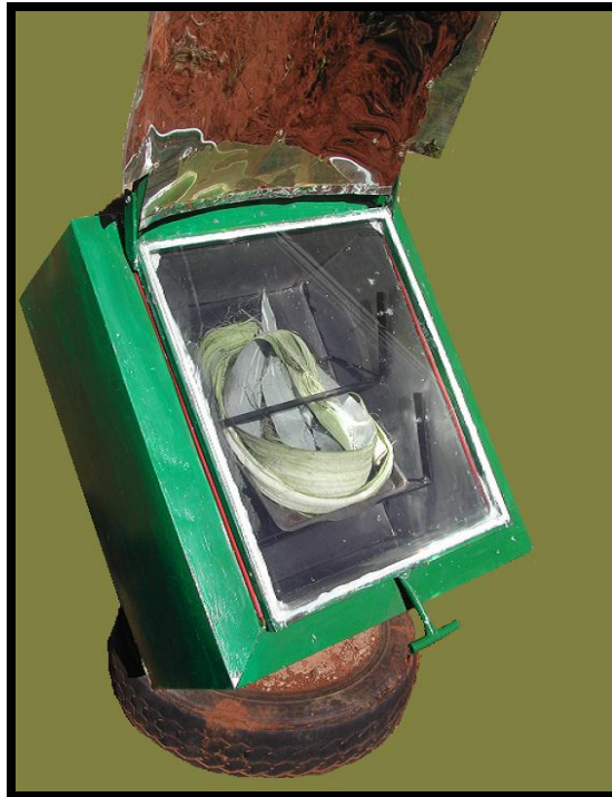
Figure 3.3 Solar baking process for partial degradation of Agave americana leaf
