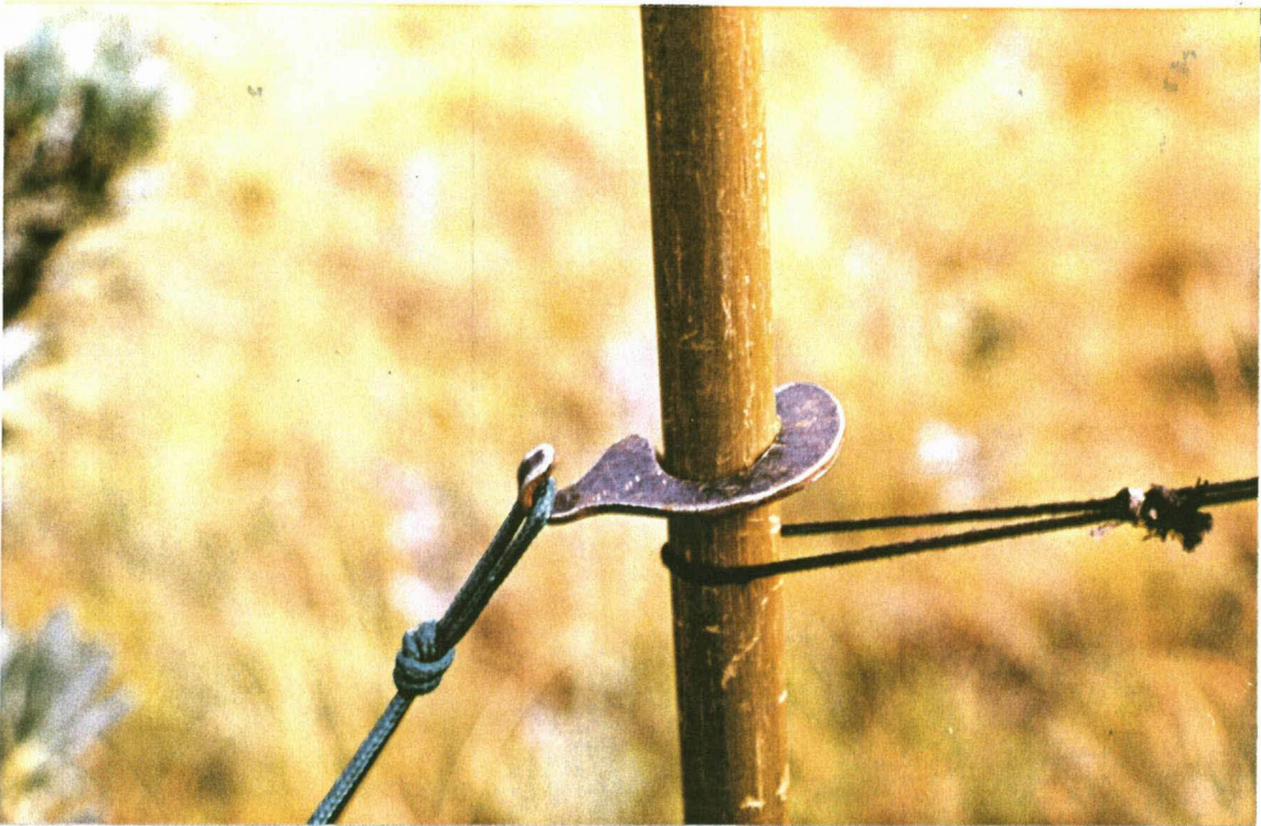
FIGURE 6: Non-slip device, which “bites” on the pole when pressed downwards, used to attach guy ropes to net poles when mist netting Gurney’s Sugarbirds.
