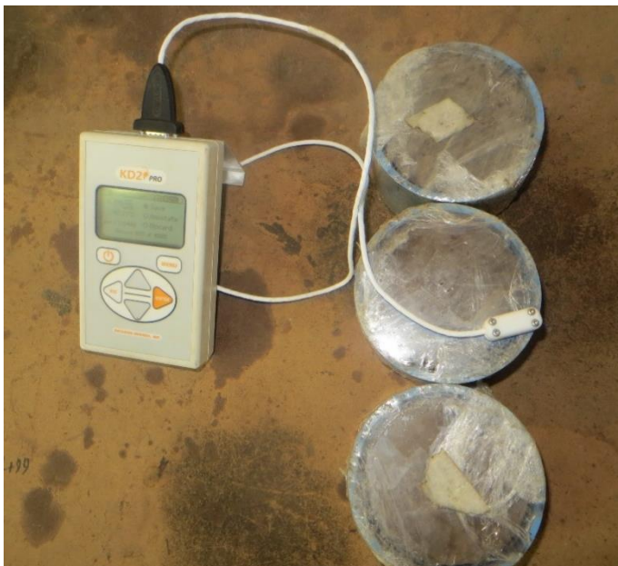
Figure 4.2 KD2 Pro analyzer measuring soil thermal properties in a room with controlled temperature (25°C).
