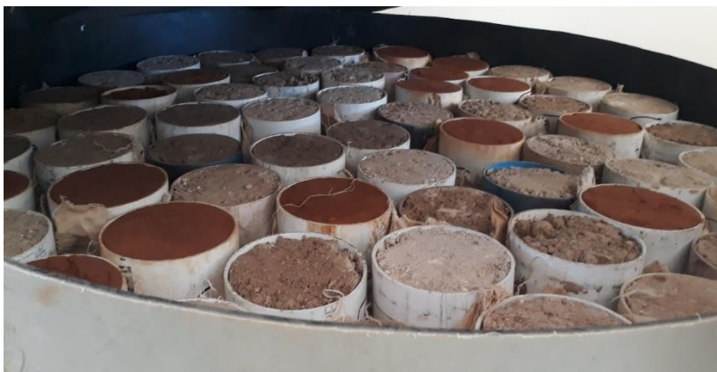
Figure 3.4 A modified drained upper limit procedure.
