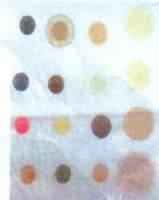
Example of a Custom Multi-Stain Monitor on CN-42 Knitted Cotton Ø = 2.5cm
