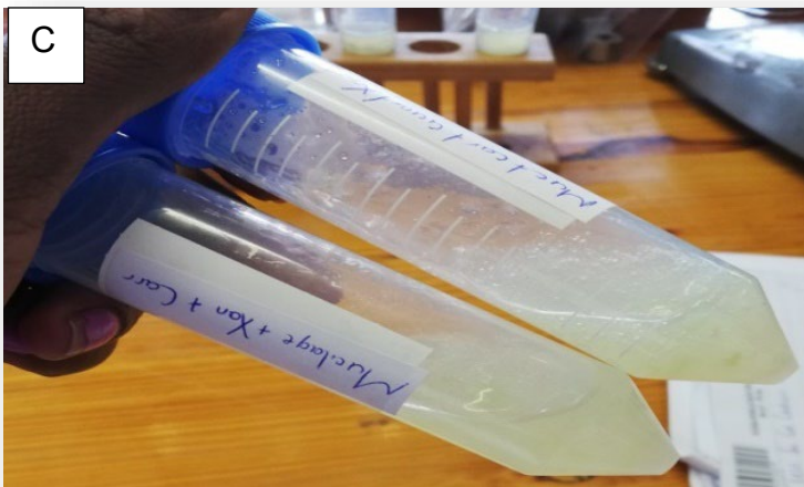
Figure 4.3 Viscous mixture formed with pH manipulation by adding NaOH and HCl (A), a mixture of mucilage with single hydrocolloids (xanthan, guar, and agar) (B) and mixture of mucilage with two hydrocolloids such as (xanthan, guar with mucilage or xanthan, agar with mucilage) (C)
