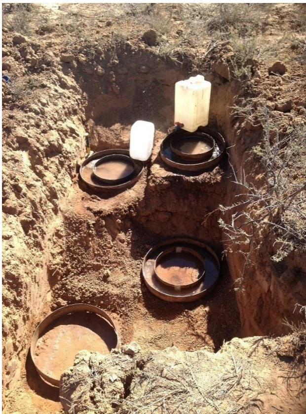
Figure 4. 1 Double ring infiltrations on Site 4.
