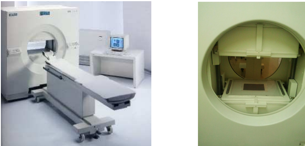
Figure 7.1: A Siemens MultiSPECT II tomographic camera with affixed transmission source.
