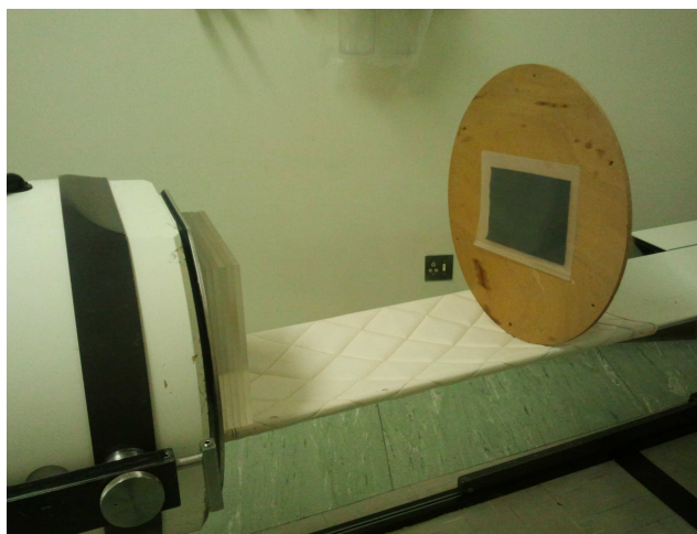
Figure 5.2: A source holder equipped with a printed transmission source supported on the bed parallel to the detector fitted with a low energy all purpose collimator. The Perspex attenuation sheets are shown on the patient support.
