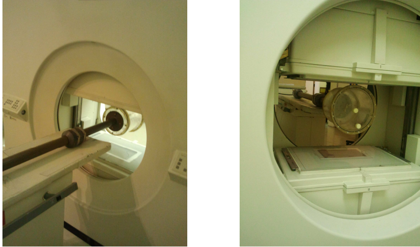
Figure 7.4: A water filled cylindrical phantom attached onto a steel pole and positioned parallel to the AOR at the COR of the gamma camera.
