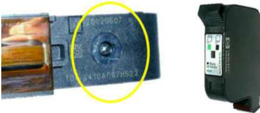
Figure 4.1: Prototype of the ink cartridge that was altered to allow for easy filling by adding a solution of black ink and Tc-99m.
