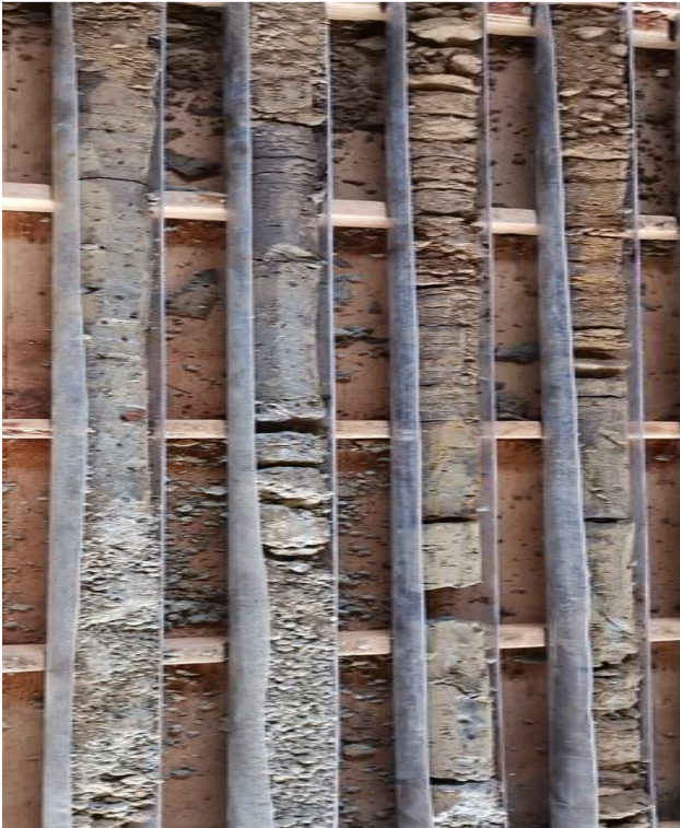
Figure 18: Example of soil cores viewed in the length of the soil profile (Ferreira, 2021)
