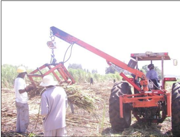
Figure 3.6 A mechanical grab fitted with a load, used to determine cane yields during harvest
