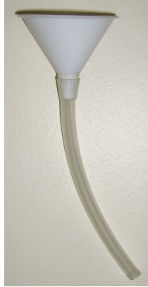
Figure 3.3 Funnel and tubing used during intubation of limestone
