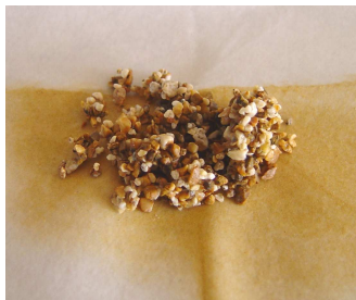
Figure 3.13 Limestone particles after filtration
