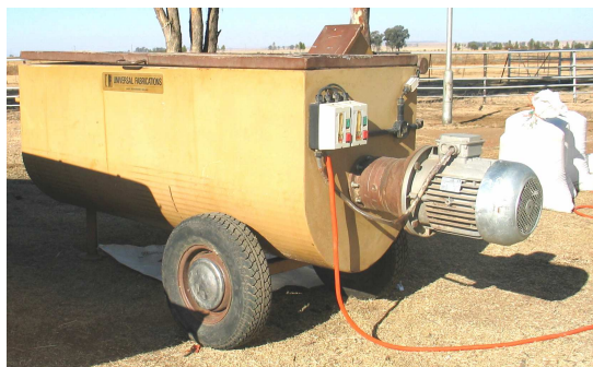
Figure 4.1 Paddle type feed mixer
