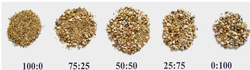
Figure 3.2 Distribution ratios of small to large (small:large) limestone particles
