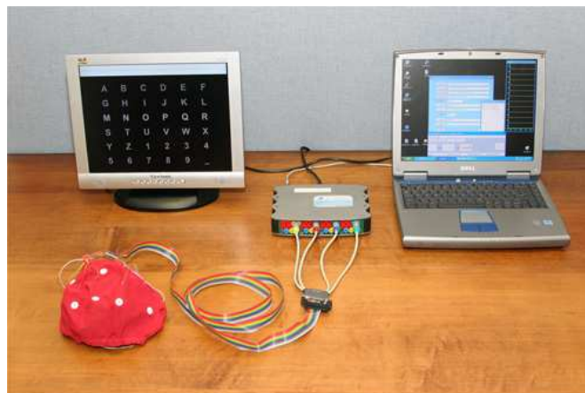
Figure 2.3: A laptop computer and redesigned cap to improve the Wadsworth BCI's portability and ease of use (Wolpaw et al., 2002).
