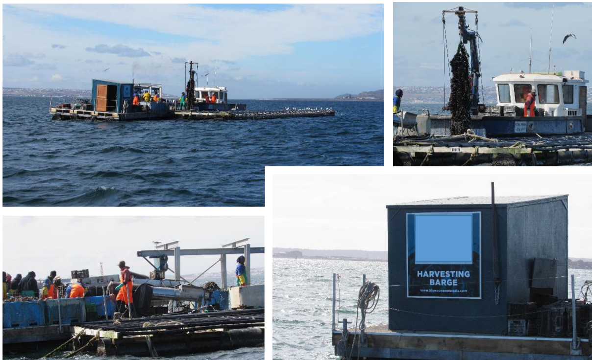
Figure 4.5: Case study 2 -boat with crane, HDPE raft and harvesting barge
