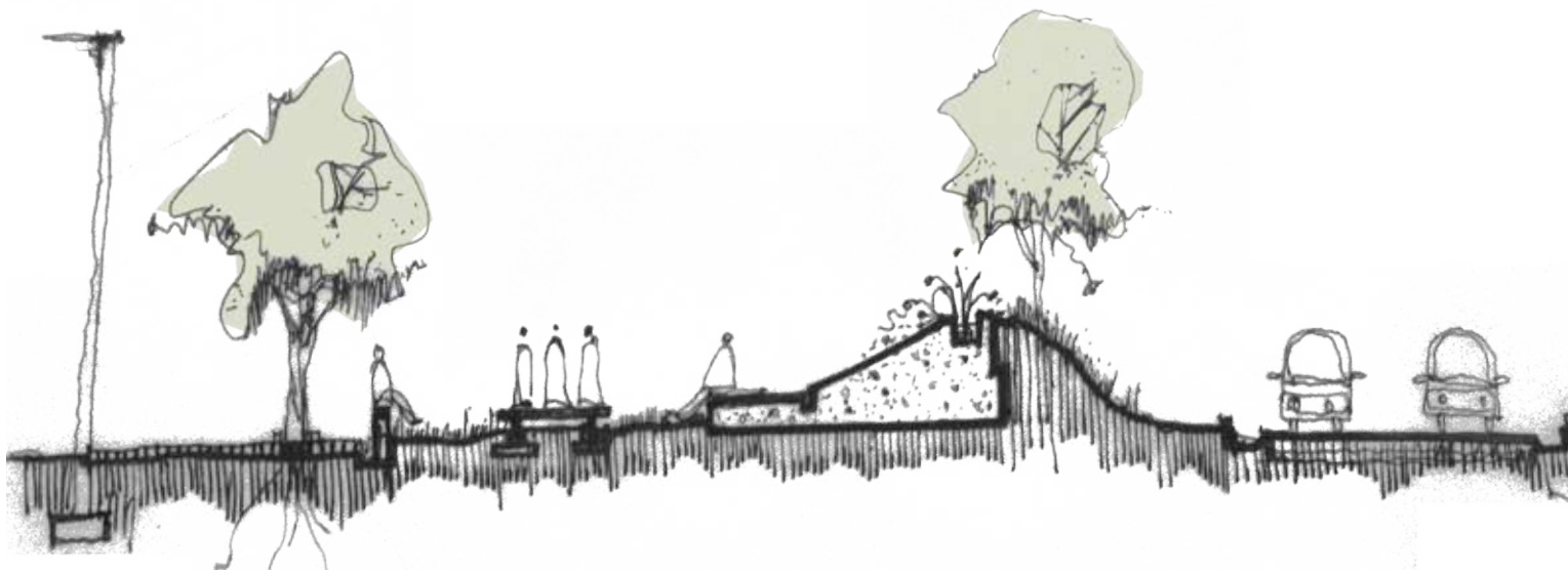
Figure 170: Noise reducing landscaping section
