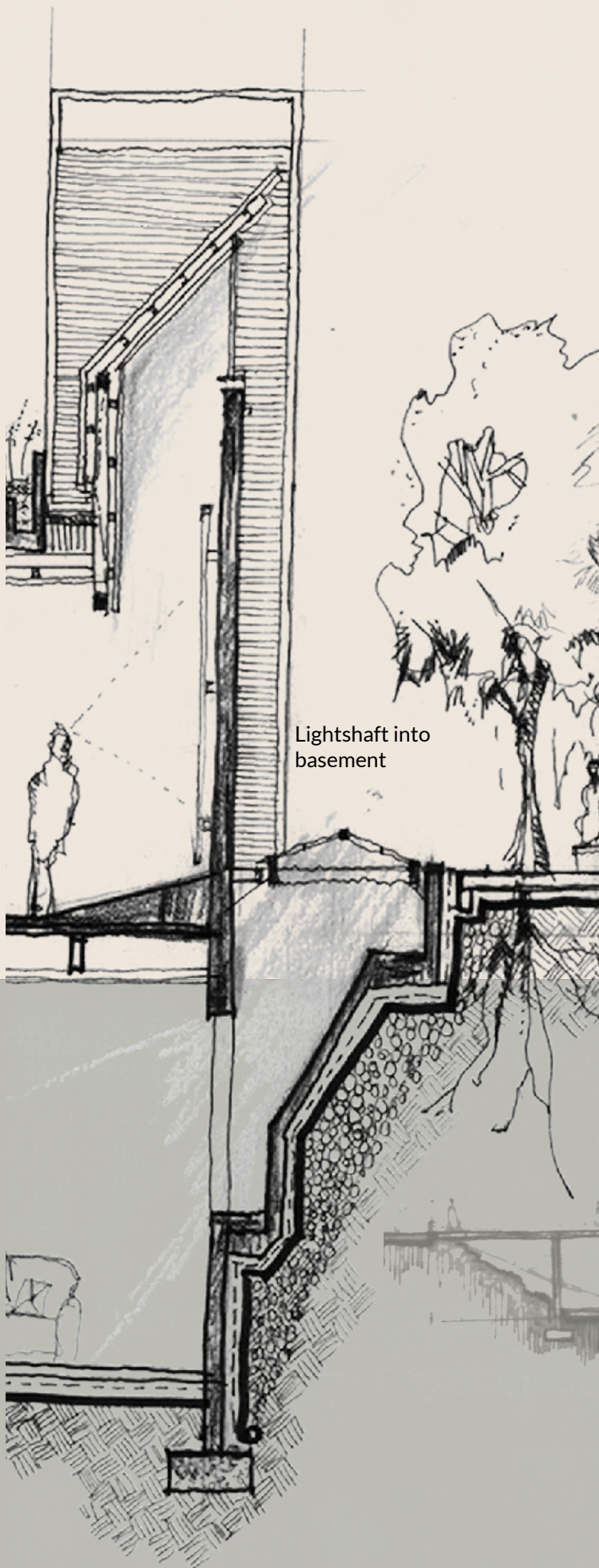
Figure 26: Detail of section showing lightshaft into basement
