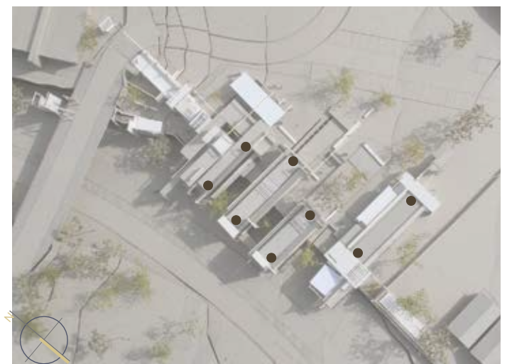
Figure 197: Placement of hvac outlets.
