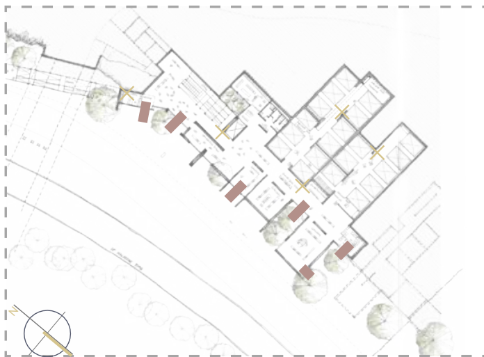
Figure 196: Fire escape routes on semi-basement.
