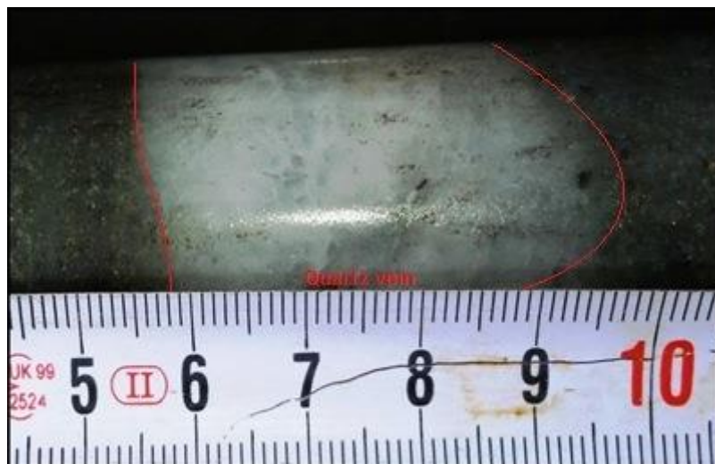
Figure 3-25: Quartz vein (thickness = 3.7 cm) encountered within drill core 2010 NE E5 X/CUT (argillaceous UF1 – Zone 2 quartzite).
