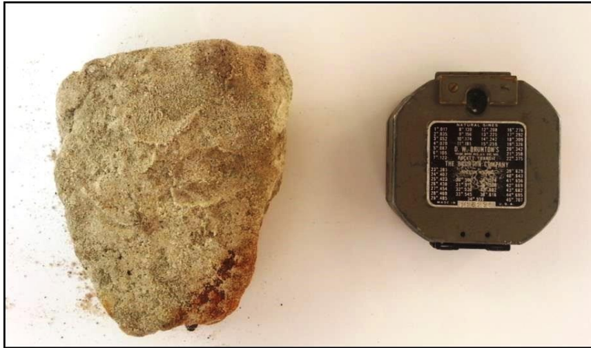
Figure 8-41: UF1 – Zone 2 argillaceous quartzite sample that was deteriorated after constantly being exposed to wet conditions. The sample was taken from 2010 NE E6 X/Cut, which is closed due to complete tunnel failure. The part of the tunnel that could be reached was extremely wet and may have possibly attributed to the natural presence of water within the vicinity. Therefore, the period of weathering is unknown. Geological compass used for scale.
