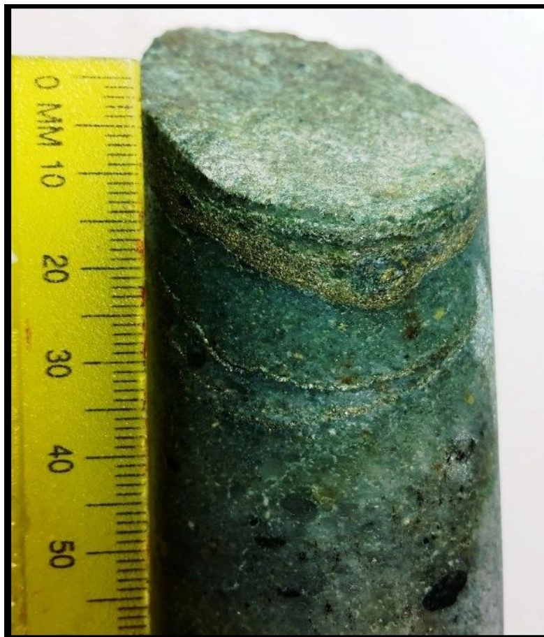
Figure 3-29: Calcite/chlorite slickenfibres encountered on the bedding surfaces within drill core 1870 NE E7 X/CUT (siliceous UF1 – Zone 2 quartzite). Pyrite bands developed on foreset beds of chlorite-stained quartzite.
