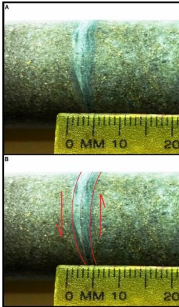
Figure 3-27: Phyllonite band (thickness = 3-4 mm) within argillaceous UF1 – Zone 2 quartzite encountered in drill core 1810 BW12 X/CUT. (A) Actual photograph and (B) interpretation of shear movement (red arrows). The BPS is also filled with secondary vein quartz (see Figure 3-19).
