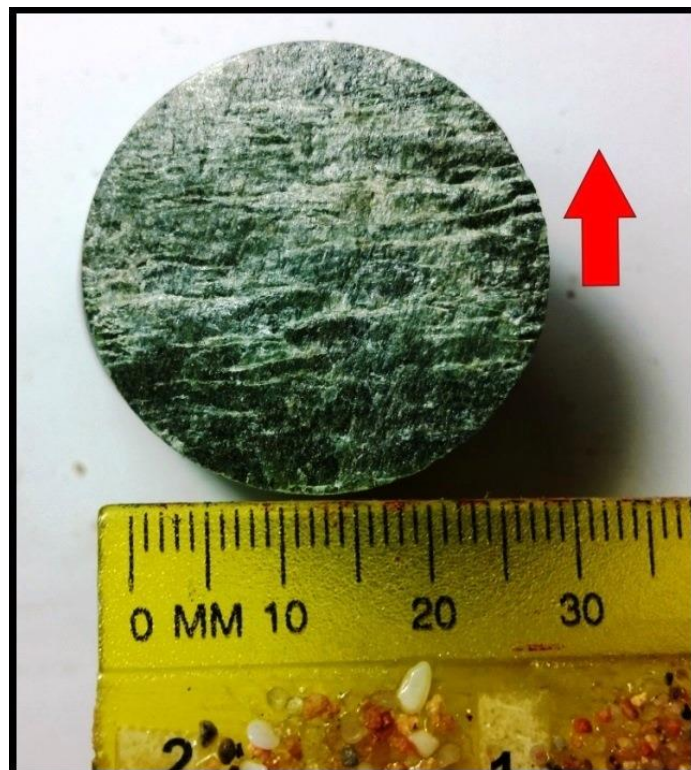
Figure 3-31: Calcite/chloritoid mineral steps encountered on fault surface within drill core 2010 SW W11 X/CUT. Shear direction is indicated by the red arrow. Growth of these minerals is associated with fault slip, which grew in the same direction as extension.
