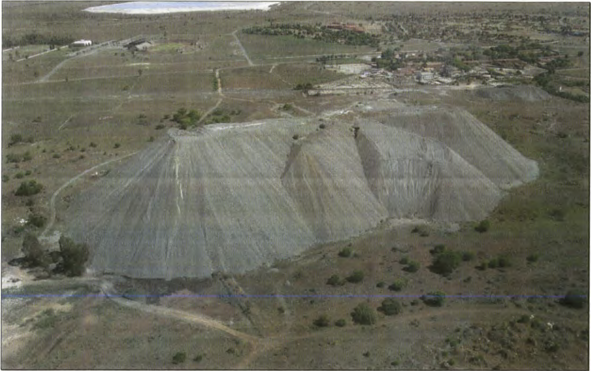
Figure 9: Example of typical Waste Rock Dump (WRD) – 3# WRD in investigation area
