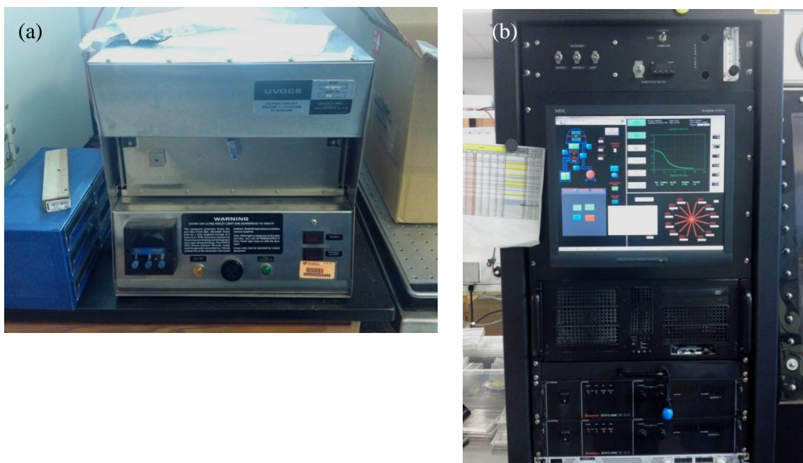
Figure 2: (a) UV ozone system used for cleaning of ITO substrate and (b) thermal evaporator used to fabricate the OLED devices.
