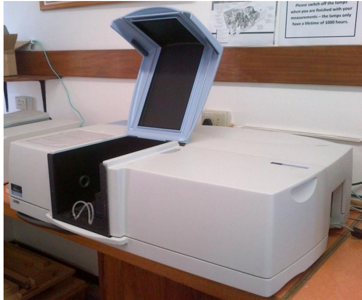
Figure 8: The Perkin Elmer Lambda 950 UV-VIS-NIR spectrophotometer.
