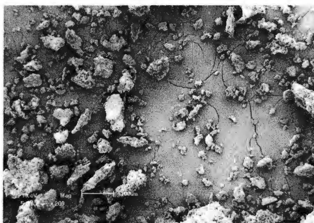
Figure 4.3 SEM image of agglomerated ZnO.
