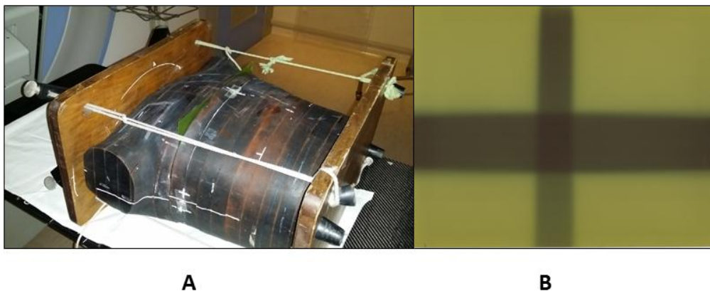
Figure 3-28: A) The RANDO ® phantom with the film inserted. B) The film after irradiation of the phantom.
