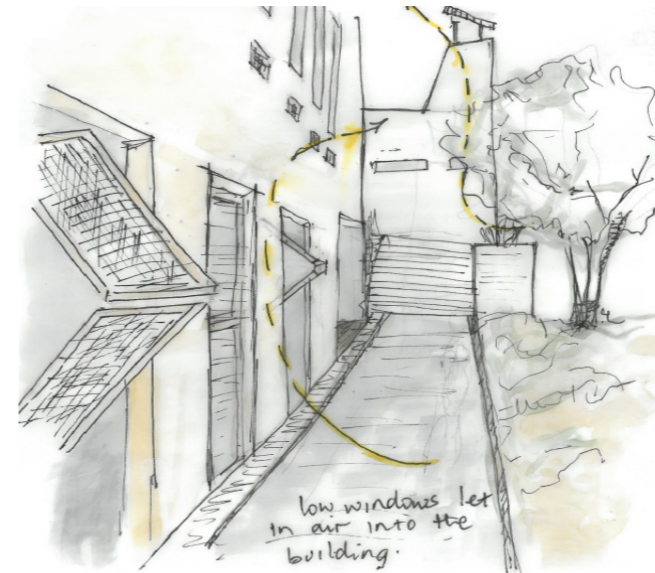
Figure 29: sketch to show low level window drawing air into the building (Author, 2021).
