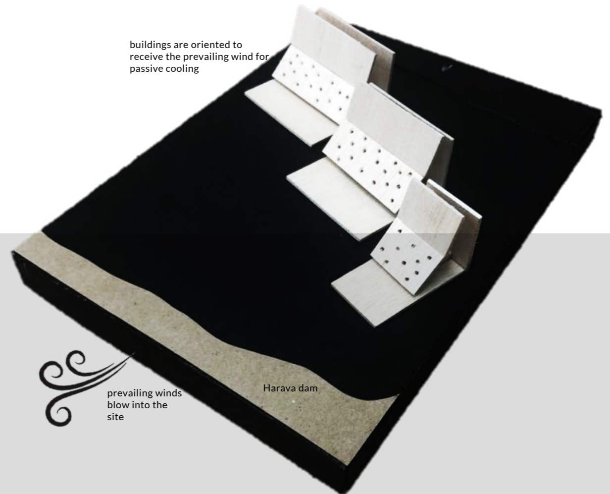
Figure 40: Biomimicry conceptual model showing the Harava Dam at the bottom and the proposal to have low apertures and chimneys for extraction of stale air from the interior spaces.(Author, 2021)
