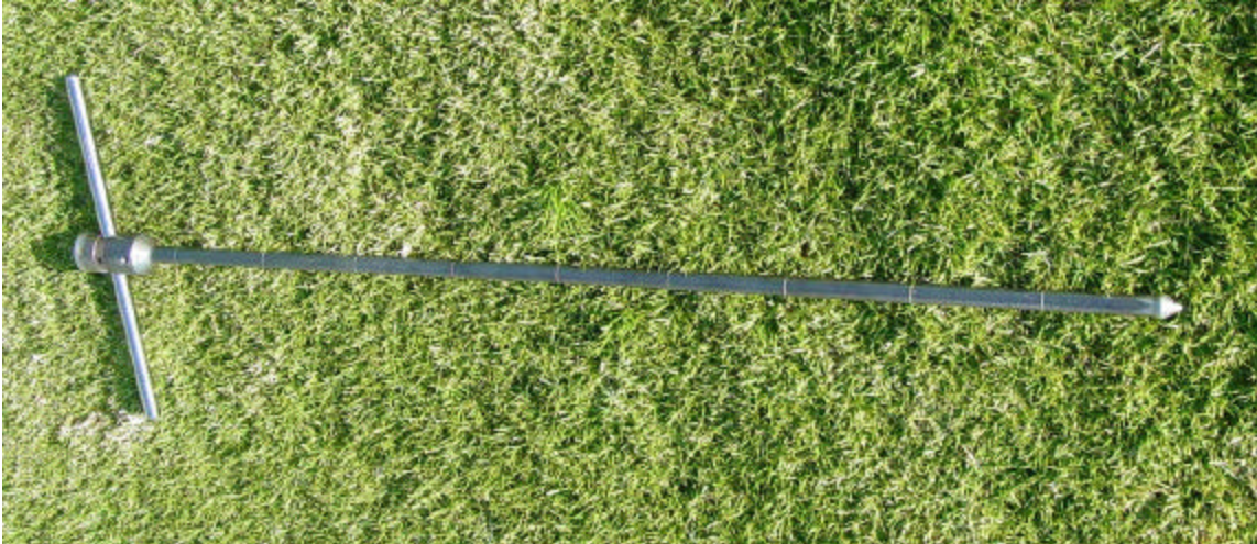
Figure 3.1 Steel probe used to estimate the effective rooting depth. The marks on the probe are at 100 mm intervals.
