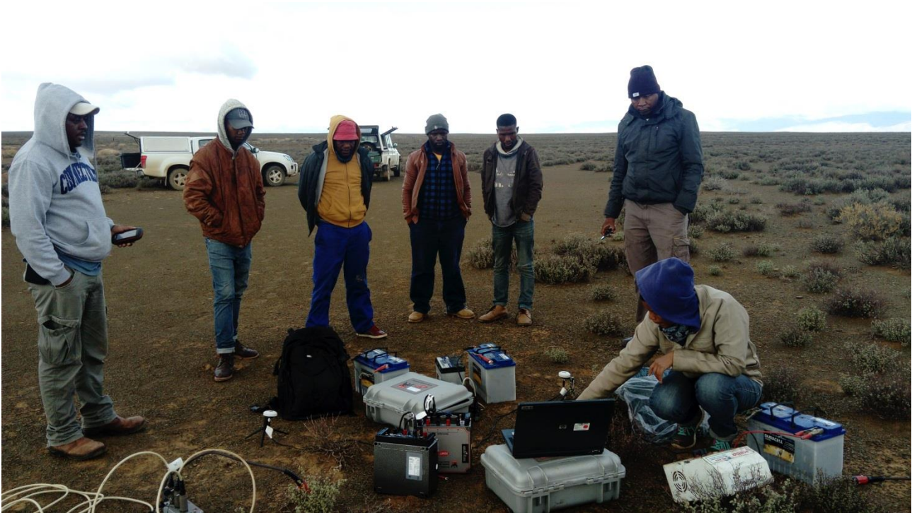
Figure 5-3: Field crew setting up the MT instrument to begin the calibration of MTU 5A receivers and the coils
