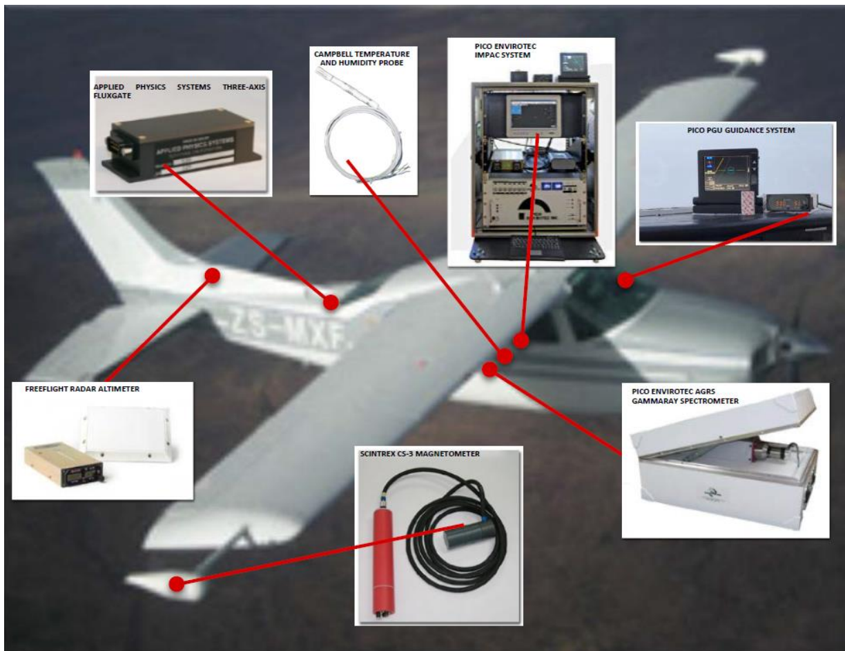
Figure 5-2: Position of instrument on Aircraft (AeroPhysics, 2017)
