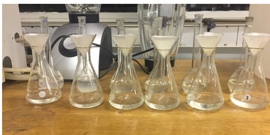
Figure 17: Preparation of samples for sugar and starch analyses
