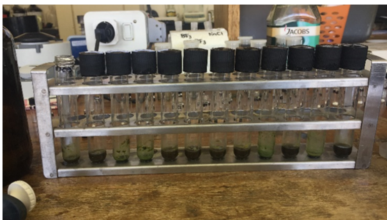
Figure 16: Transesterification of various nopalito cultivars in progress
