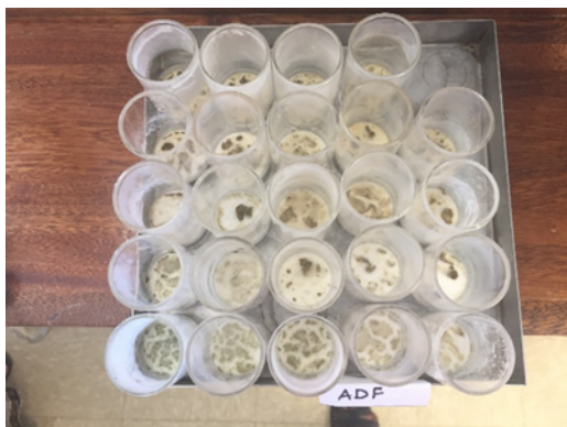
Figure 14: Various nopalito samples being investigated for Acid Detergent Fibre content
