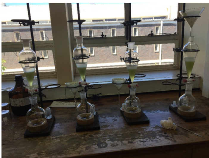
Figure 15: Extraction of total lipid content in various nopalito cultivars in progress
