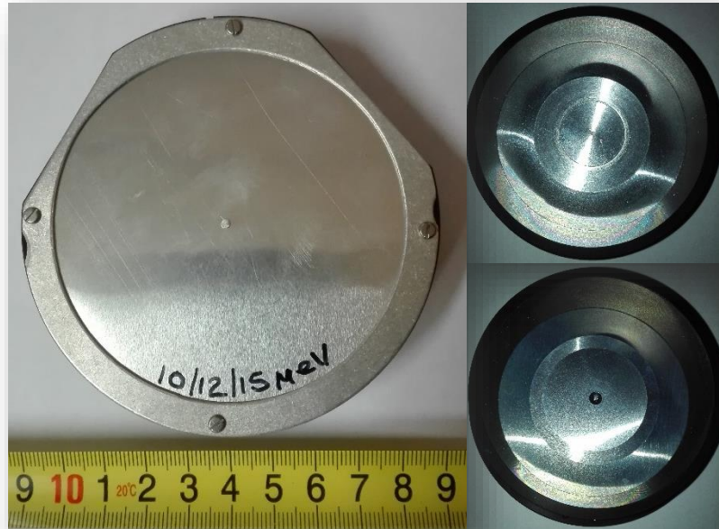
Figure 3-1: On the left side a bottom view of the high-energy scattering foil is given. Both the images on the right side represent a top view of the scattering foils, illustrating the difference in the number and radii of foils used within each scattering foil holder. The top right image is the low-energy scattering foil and the bottom right image is the high-energy secondary scattering foil.
