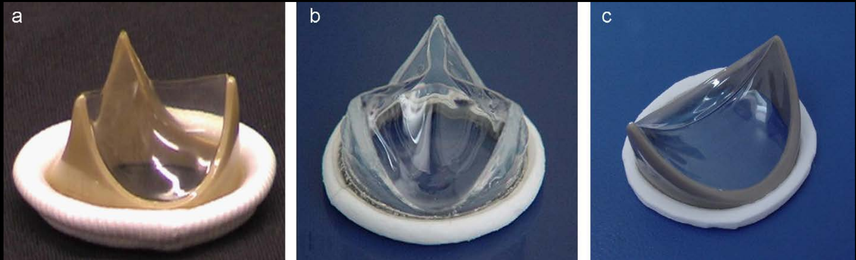
Fig. 8. Polymeric heart valves: (a) a frame machined from polyetheretherketone (PEEK) and coated with a thin layer of leaflet polyurethane. Leaflets of a commercially available polyetherurethane suitable for animal implantation (Estane 58315, BF Goodrich, Westerlo-Oevel, Belgium) were dip-coated onto the frame. This valve design has achieved durabilities in excess of 400 million cycles (10.5 years) during in vitro fatigue testing [162]; (b) and (c): polycarbonate urethane (PCU) tri-leaflet and bi-leaflet valves intended for the aortic and mitral positions. These particular designs achieved in vitro durabilities of up to 600 million (15.8 years) and 1 billion (26 years) cycles, respectively.
