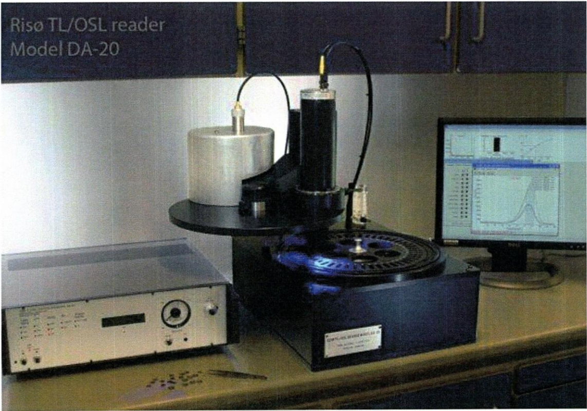
Figure 3.29: A Risø model TL/OSL-DA-20 Luminescence Reader [55].
