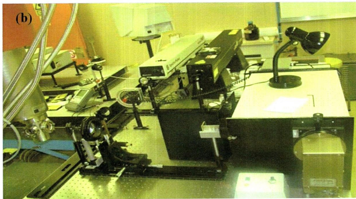
Figure 3.20: (a) Schematic diagram of the PL system (b) PL system used to investigate the luminescent properties of phosphors.
