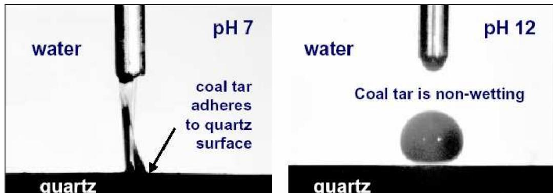
Figure 7: Photomicrographs of a coal tar-water system and aqueous pH 7 and pH 12. (Needle size for scale: o.d. = 0.52 mm). (Barranco and Dawson, 1998)
