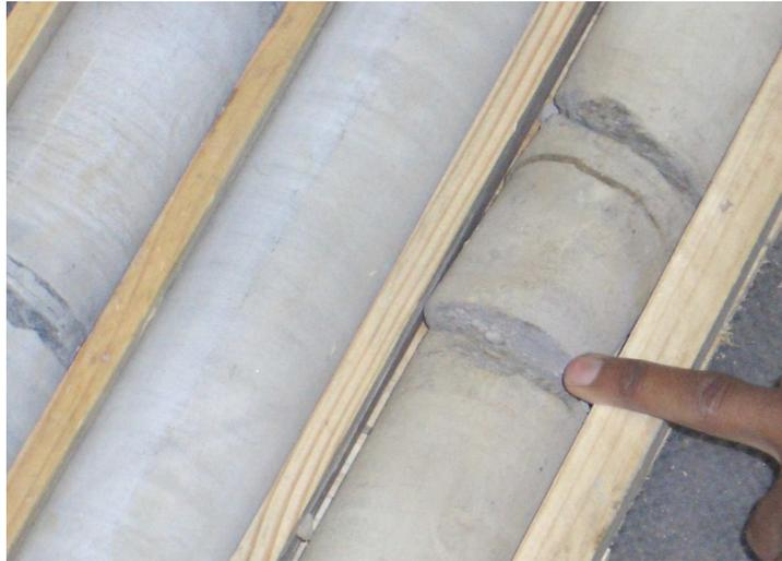
**Figure 5-17: Mode 1 fracture in DC2 at 20.96 m.**
