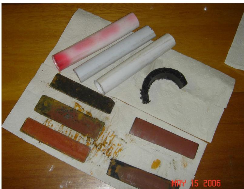
**Figure 5-95: Effect of TCE (dyed red) on casing material after 18 months of exposure.**
