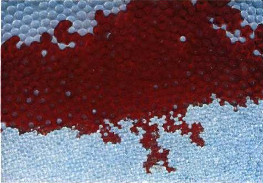
**Figure 3-5: Example of a two-layer bead medium, initially saturated with water. Entry of smaller pore space by DNAPL only after sufficient pressure as result from pool height (From Schwille, 1988).**
