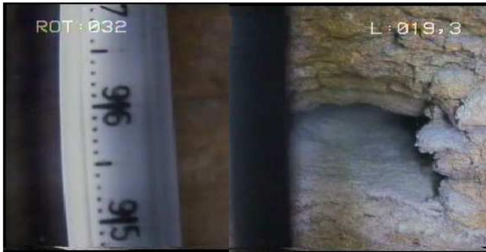
**Figure 5-13: Video camera image of Borehole D3 with accurate depth measurement of the fracture.**
