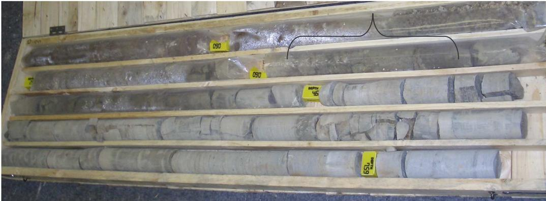
**Figure 5-16: Vertical fracture in DC1 at ~5 m (top) and mode 1 fracture at 21 m (bottom) in DC1.**
