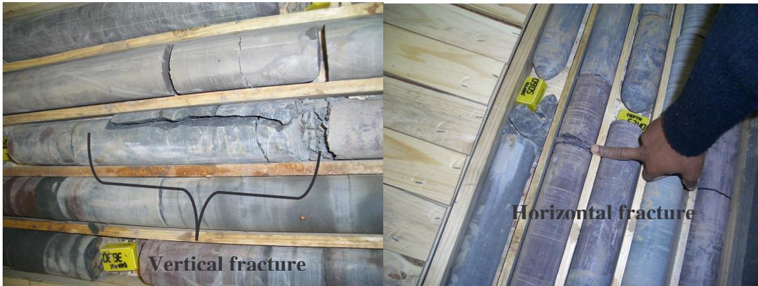
(A) Vertical fracture around 36 m in EC1
