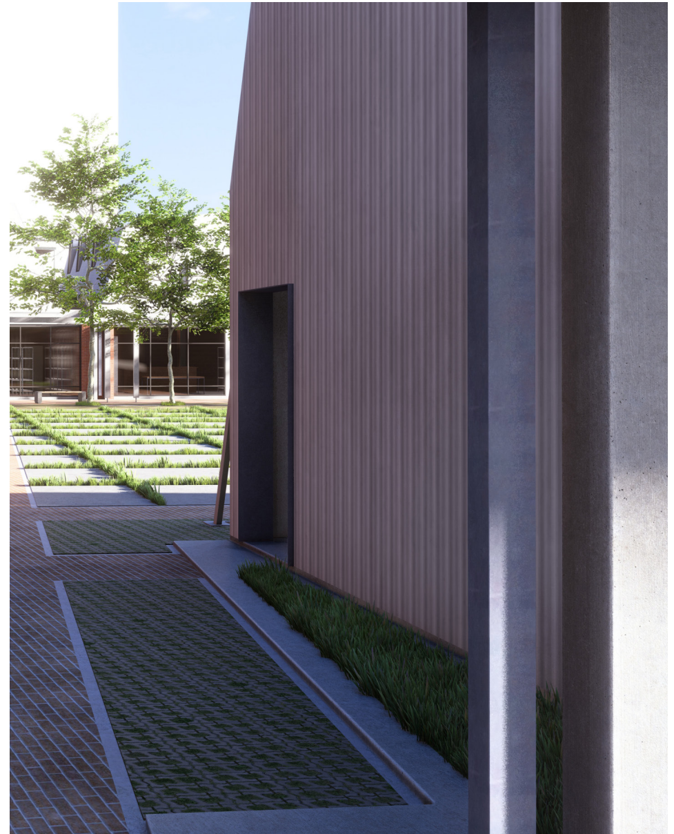
Figure 198: Permeable stormwater management system (Author, 2023).
