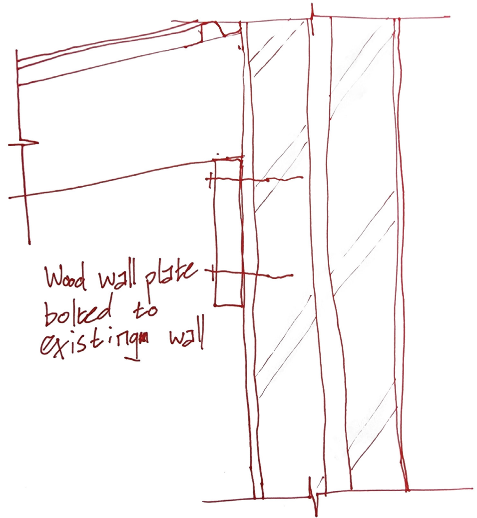
Figure 193: Detail of new connecting to old (Author, 2023).
