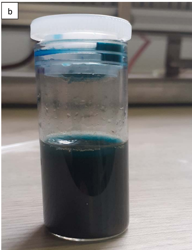
Figure 3.14: (a) Shows initial and final MB solutions, (b) during the sonication process, and (c) removal of magnetite nanoparticles using neodymium magnetic, after 480 min of sonication.
