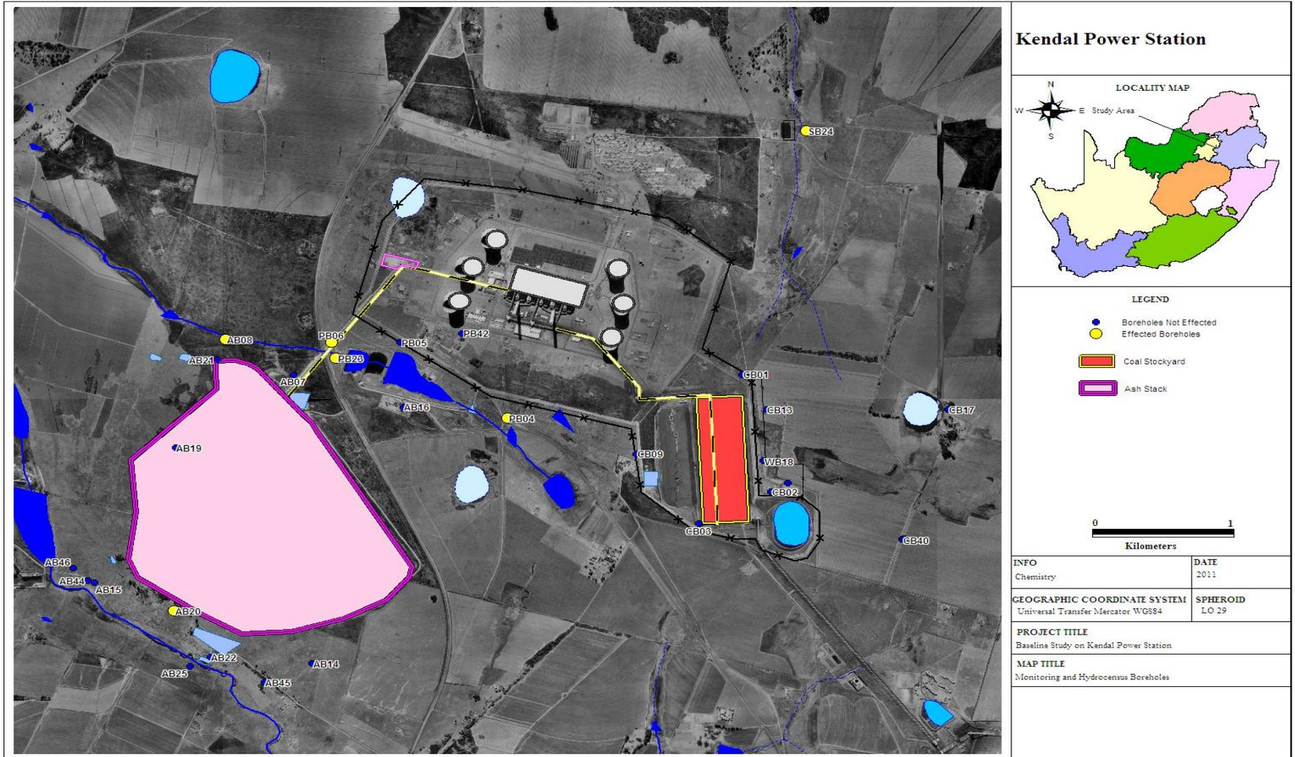
Figure 29. Boreholes exceeding average Na concentrations of hydrocensus boreholes.
