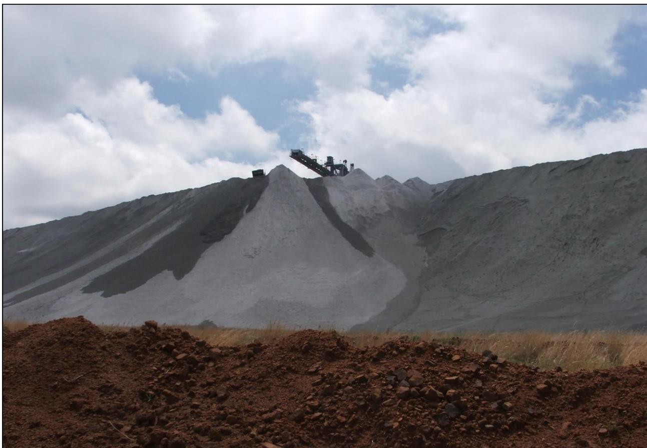
Figure 5. Conveyor belt ash disposal.
