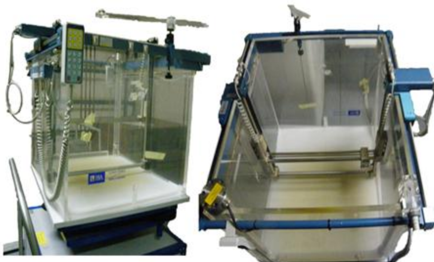
Figure 3.5: Water Tank used for physical measurements
