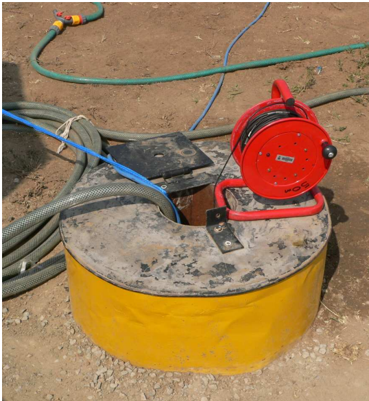
Figure 3-21 Set-up around the borehole and the flowcell.
