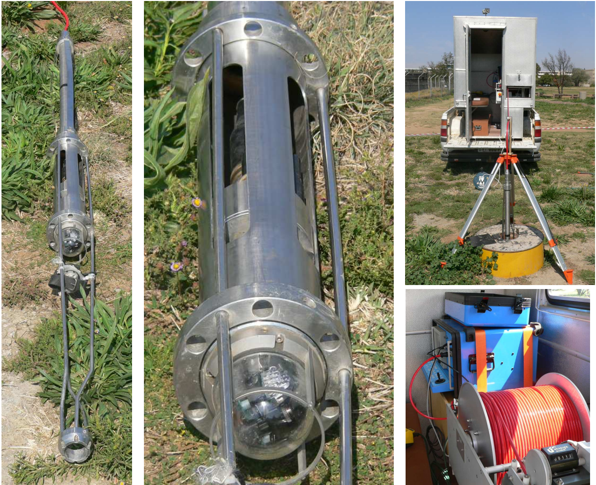
Figure 6-19 Set-up of the borehole video camera (UO20 and UO14).
