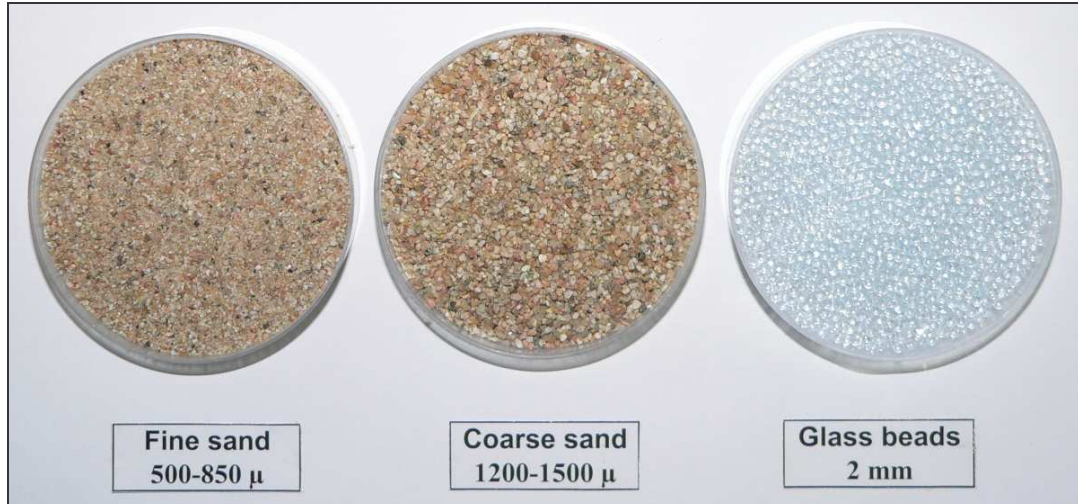
Figure 4-3 Packing material - fine sand, coarse sand, and glass beads.
