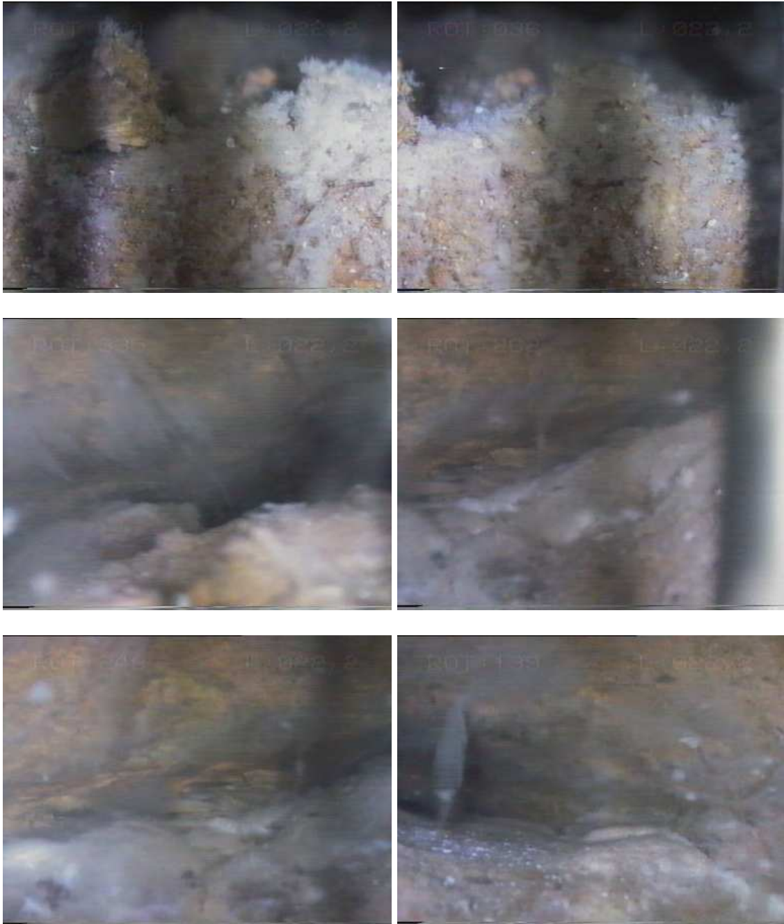
Figure 6-21 Borehole video camera observations (Day 16, UO7, 22.8. m). (White material is biomass).
