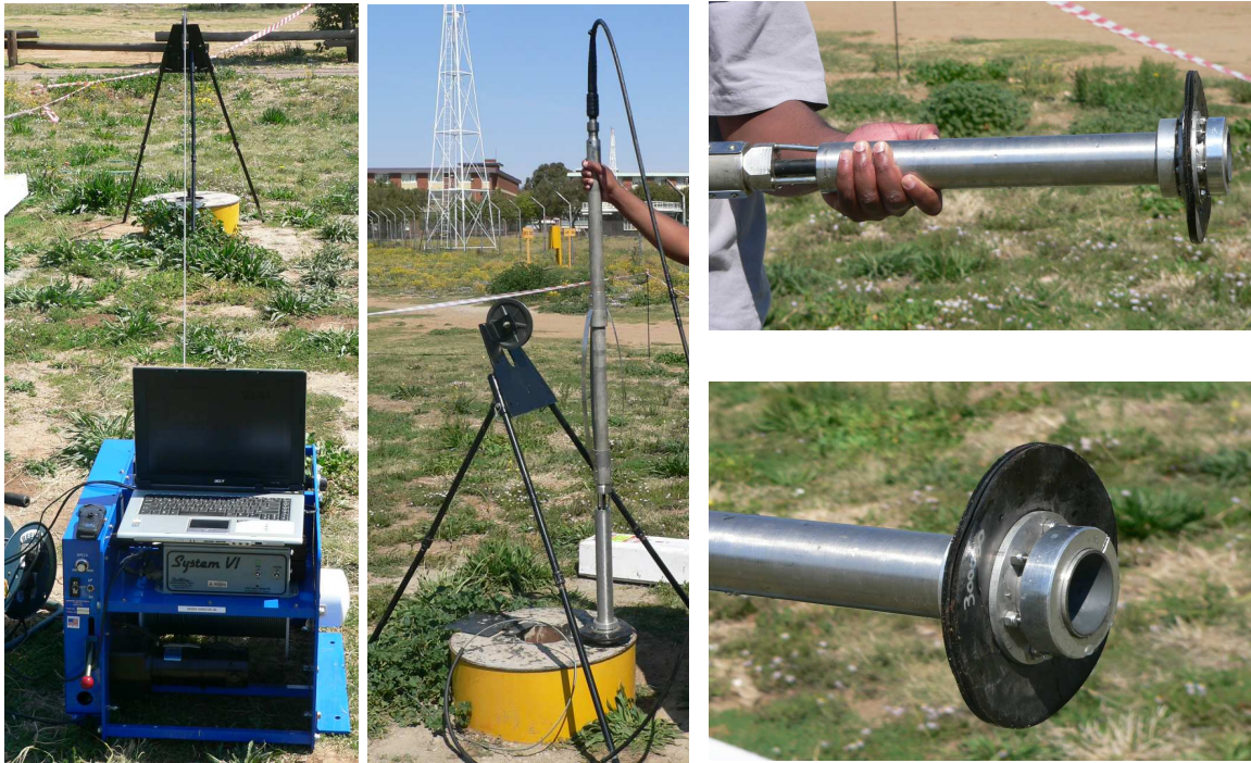
Figure 6-16 Set-up of the flowmeter (UO20 and UO14).
