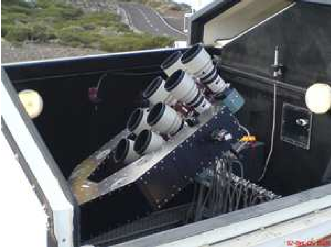
Figure 5.2: A picture of the superWASP observatory showing the eight cameras ( Adopted from http://www.superwasp.org ).
