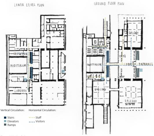
Figure 239: Circulation (sketch derived from architects drawings)
