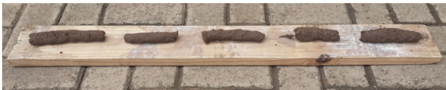
Soil shaped in a roll of 3cm in diameter and 15cm in length (Photograph: author).
