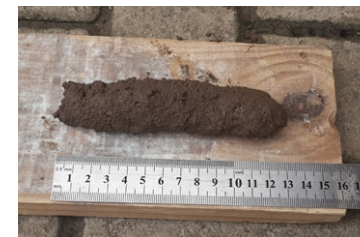
Pieces broken off and measured to perform cigar test (Photograph: author).
