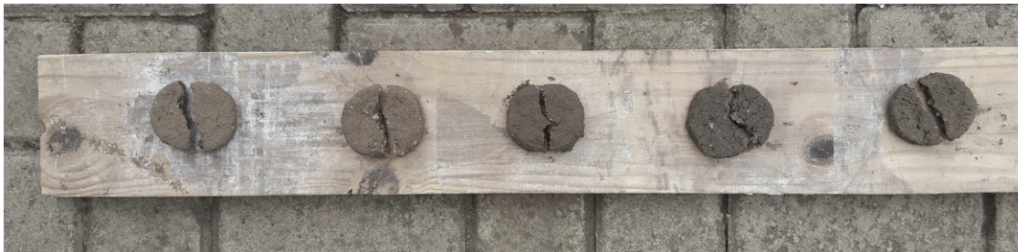
Different 'biscuits' after strength test (Photograph: author).
