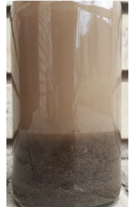
Layers visible during the bottle test (Photograph: author).
