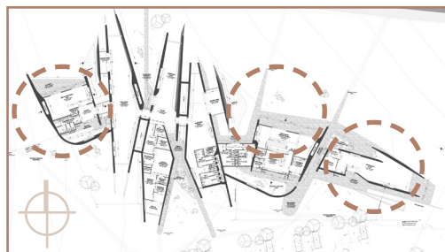
Figure 3.2.12: location of secondary functions with orientation of long facades opening up to south and north
