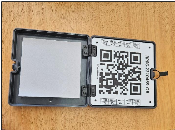
Appendix B: The calibration reflectance panel from MicaSense.
