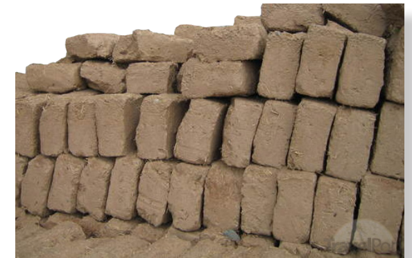
Figure 134: Adobe bricks used as infill material (TravelPod, [n.d.]: Online)
