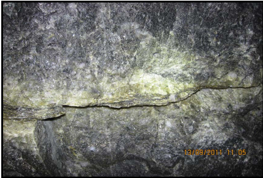
Fig.2.11 A ductile shear zone below the UE7 conglomerate. Microscopic carbon nodules are present within this phylonite.
