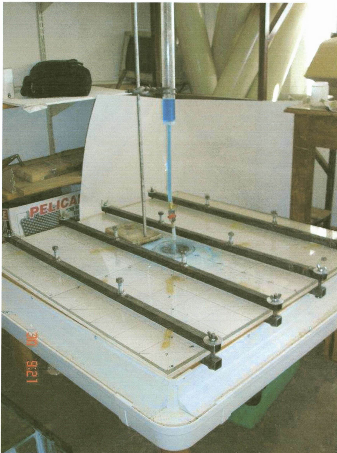
Figure 2.7. Laboratory apparatus for the fracture aperture determination experiment: Note the clamped thickness gauge blades to create the fracture aperture between two circular 100cm x 100cm square Perspex plates.
