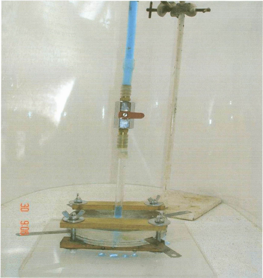
Figure2.6. Laboratory apparatus for the fracture aperture determination experiment using blue colored water, Note the clamped thickness gauge blades to create the fracture aperture between two circular 100mm diameter Perspex plates.
