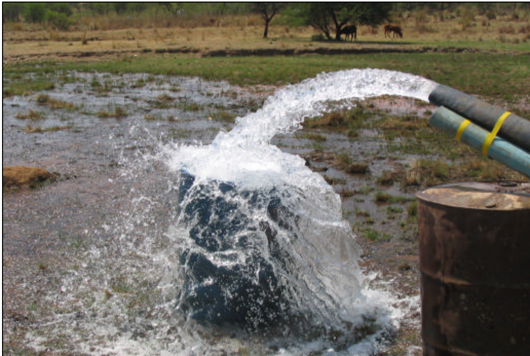
Figure 17 Borehole visited on the Nebo Plate au. After switching off the pumps this borehole had artesian flow of 3 l/s
