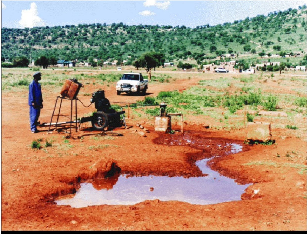
Figure 21 Ponding and soil erosion as a result of poor borehole development and management
