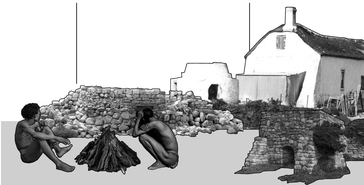
Figure 83: Kiln development: Bonfire, pit kiln, beehive kiln, cat kiln (Walton, 1965: 23) (edited author).
