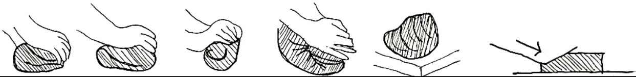
Figure 87: Drawing of the wedging process (author).
