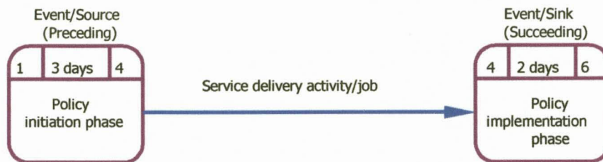
Figure 5.2 represents an arrow network diagram consisting of preceding and succeeding events.
